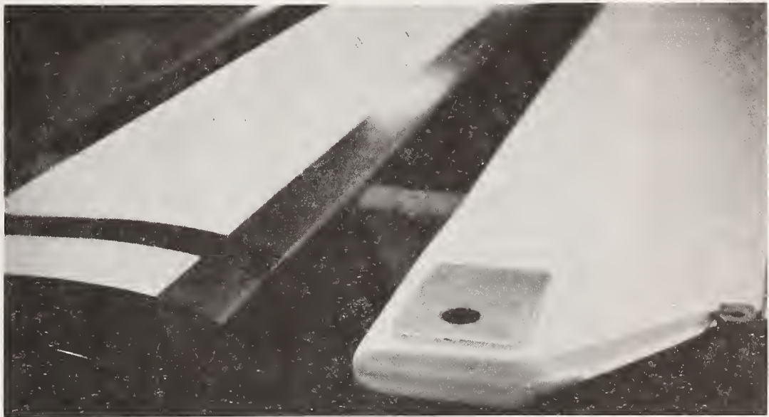
Fig. 6a and b Main Rotor Blades-Glass/Epoxy
