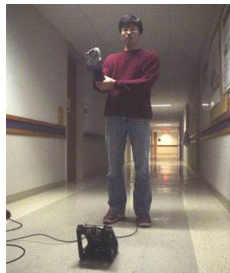
Figure 1: Using the Gestural Joystick to operate a commercial Inuktun robot.
