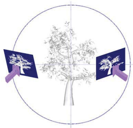
Figure 3. The demonstration for capturing several silhouettes from defined positions on the surface of bounding sphere.
