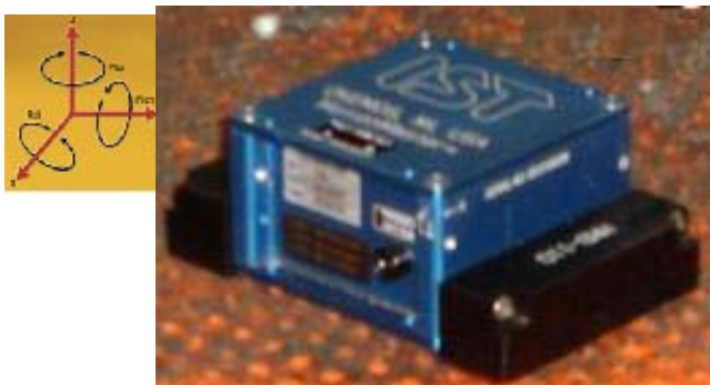
Figure 3 An Accelerometer with Embedded Data Logging Capabilities
