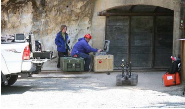
Figure 6: Robot operator positioned at the entrance to the Hazel-Atlas mine tunnel. The robot was operated in a non-line-of-sight condition more than 100 m inside the tunnel.
