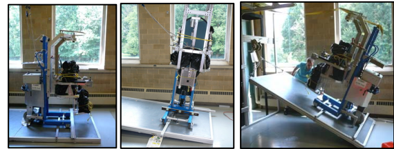
Figure 3: Photos of example test configurations, including: (left) forward, (middle) lateral, and (right) rear configurations.
