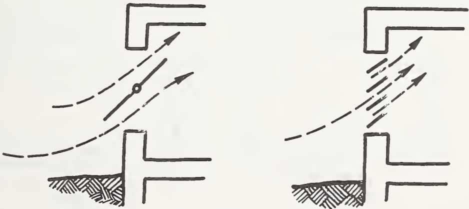
Figure 22. Section Through Horizontal Pivoting Windows
