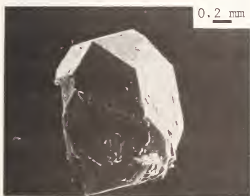
Figure 4. Single crystal of flux-grown tetragonal \text{K}_{1+x}\text{Al}_{1+x}\text{Si}_{1-x}\text{O}_4 . Note flat faces suitable for semi-quantitative analysis. 20 kV, 0^\circ tilt.
