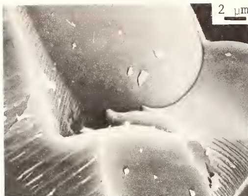
Figure 9. Liquidus studies - experiment above liquidus. K_{36}S_{64} , 1658°C. Fracture surface, no evidence of crystalline phases in glass. 20 kV, 45° tilt.
