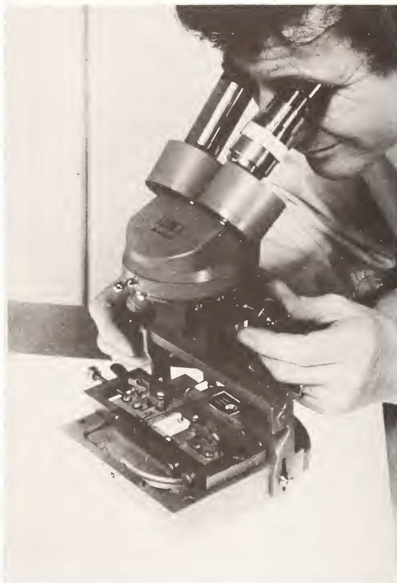
Figure 4 : Measuring the number of courses per centimeter of an explanted prosthesis with the pick counter in transmitted light.
