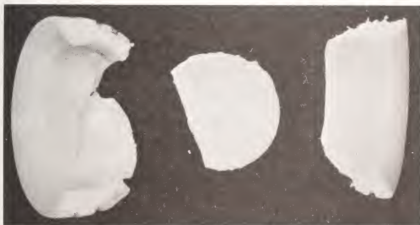
Figure 5: Worn and fractured polyethylene acetabulum described by Salvati et al. [51].
