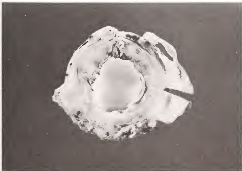
Figure 2. Atrial view of a Beall model 104 mitral valve with marked sewing ring fabric wear. Implanted for 6.5 years, note loss of neointima from frayed fabric in the inflow tract.
