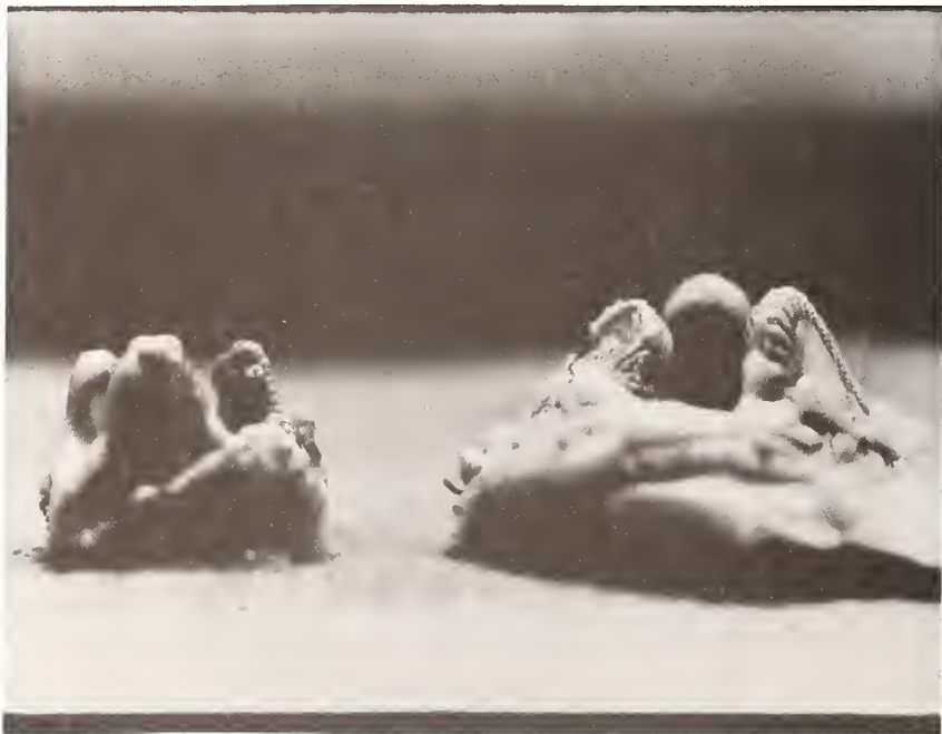
Figure 20. Same two recovered valves. This figure shows the phenomena of "creep" (drooping inwards) of the stents of the mitral valve.
