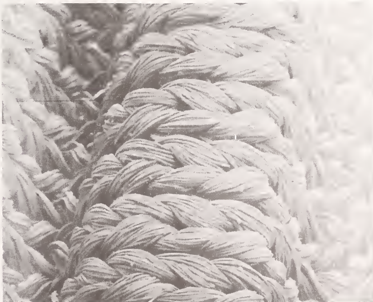
Figure 8.08 : (B74) Internal view of a Weavenit prosthesis with undamaged fabric structure and preserved crimp after 3 days in-vivo.
