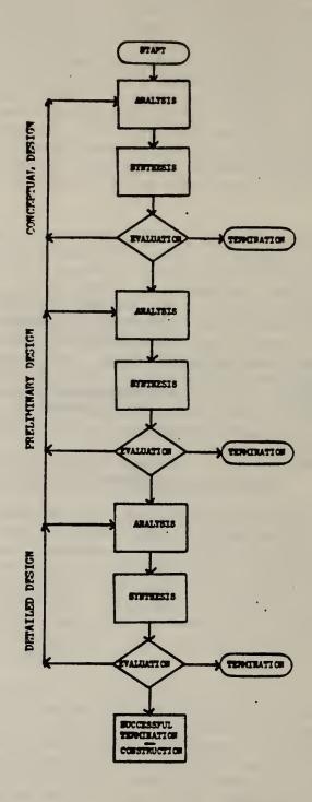
Figure A.3. Iterative engineering design process
