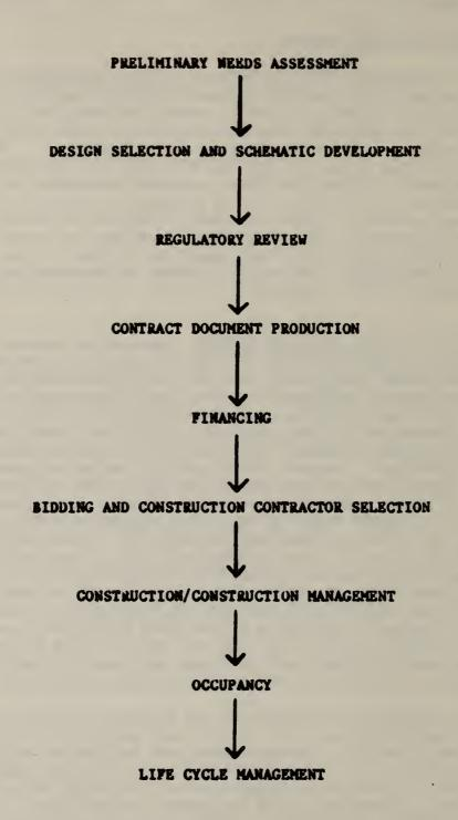
Figure A.1. A simplified overview of the building delivery process
