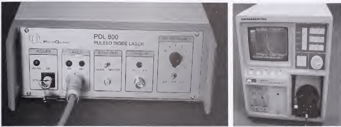
Fig. 8: Fast laser pulse source and Optical Oscilloscope Hamamatsu OOS-01/VIS
