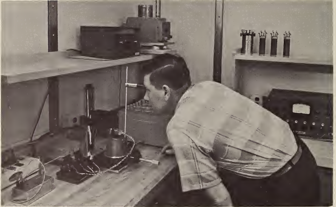
Fig. 1 Test Set-up for Precision Measurements of Resistivity of Silicon Wafers by the Four-Probe Method.
