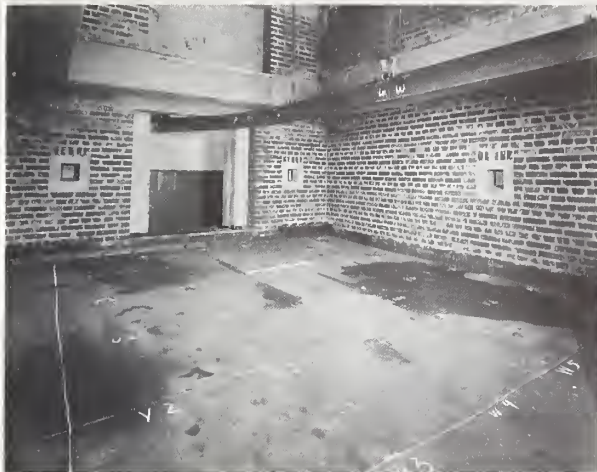
FIGURE 3.—Upper furnace space; bare steel-deck floor.
