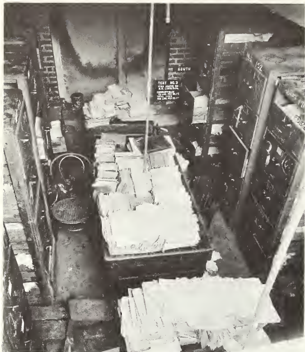
FIGURE 6.—Burnout space above the floor; thermocouples contained in suspended iron pipes; showing arrangement of combustible materials.
