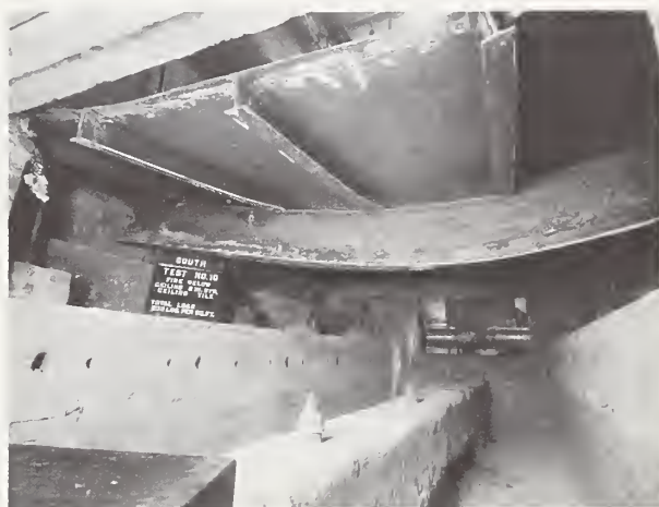
FIGURE 14.—Deformation of girder and cantilever beams after 5-hr fire exposure (ceiling and girder covering removed).
