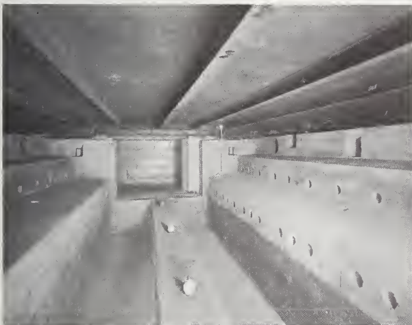
FIGURE 4.—Lower furnace, steel deck-and-beam floor in place, prior to installation of protective ceiling.
