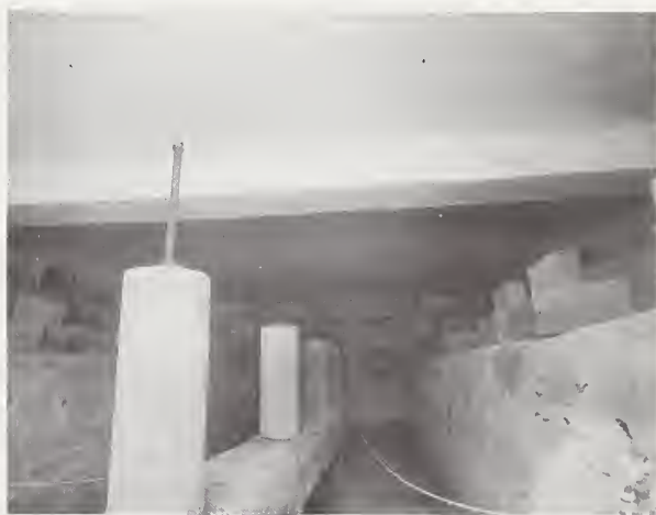
FIGURE 5.—Lower furnace showing iron pipes for protection of furnace temperature-measuring thermocouples.
