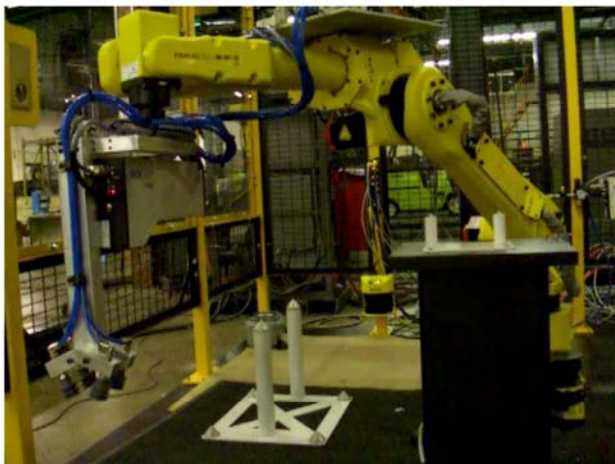
Calibrating robot with SICK 3D reference tool
