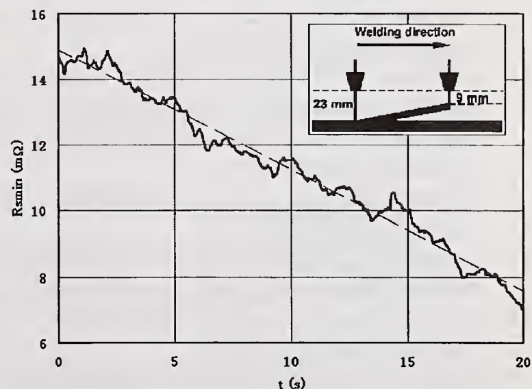
Figure 14. Sensor output during uphill welding ( I=180A , U=19V , v_d=5.2m/min , MS wire \varnothing 1.2 mm, CP mode, K_I=60kA/s )
