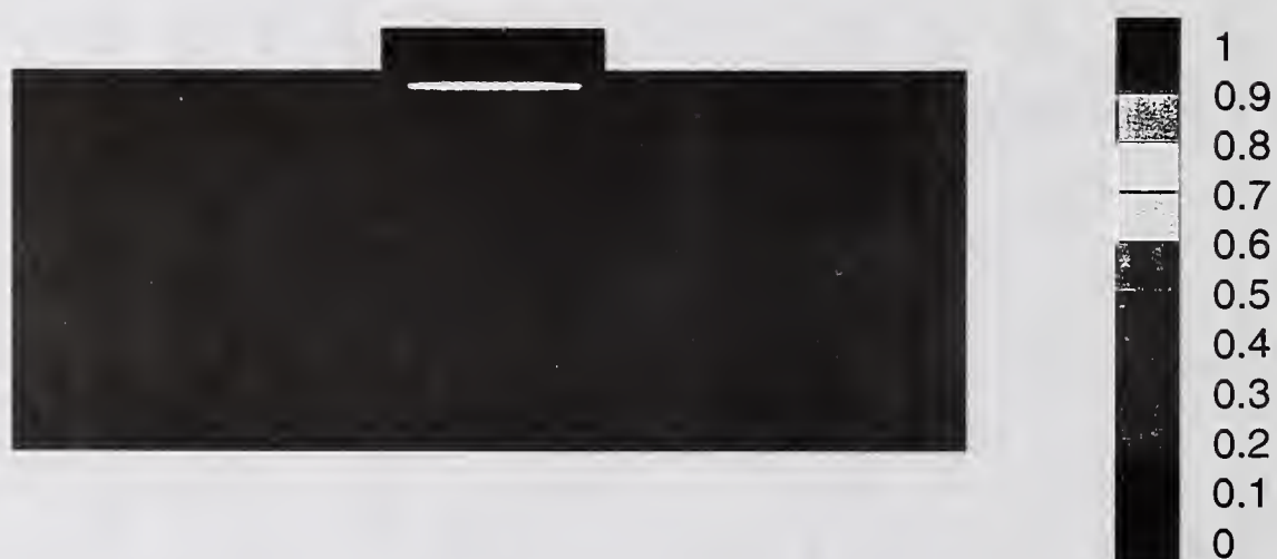
Figure 6 Predicted martensite distribution (volume fraction)
