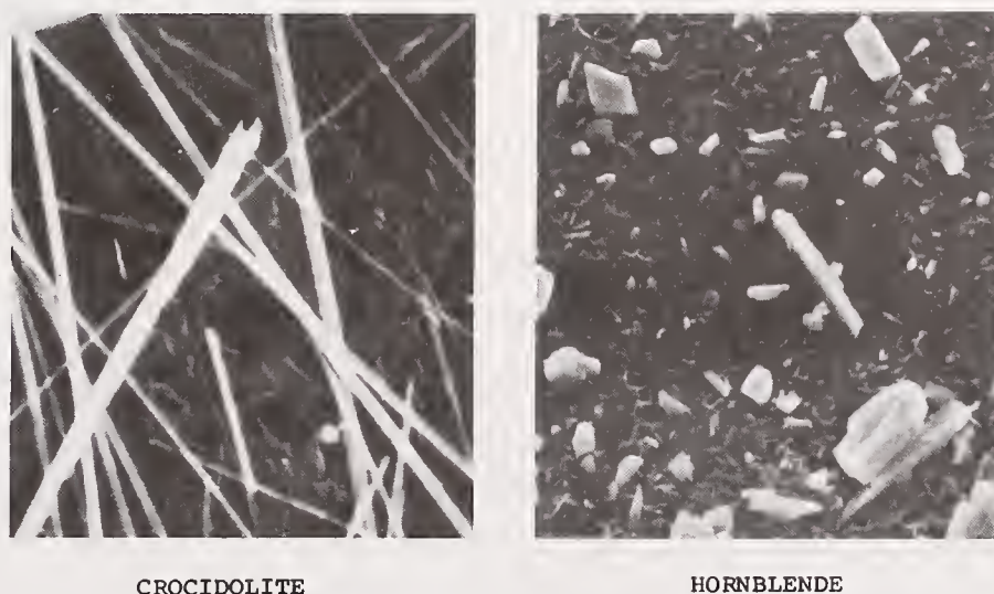
Figure 12. Scanning electron micrographs of crocidolite fiber and fragments of hornblende.
