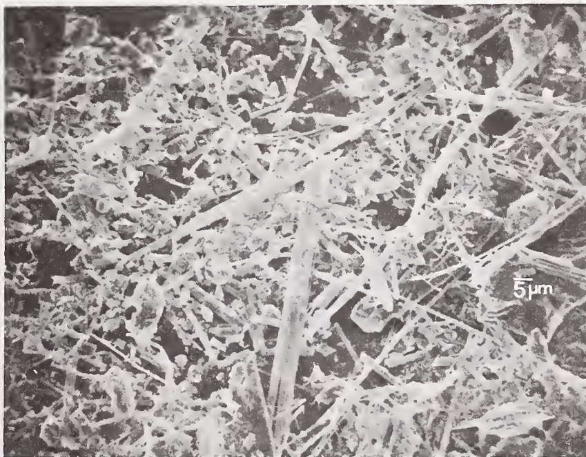
Figure 2. Talc-Fiber No. 1 from International Talc Co. Analyzed as asbestiform tremolite with minor talc content.
