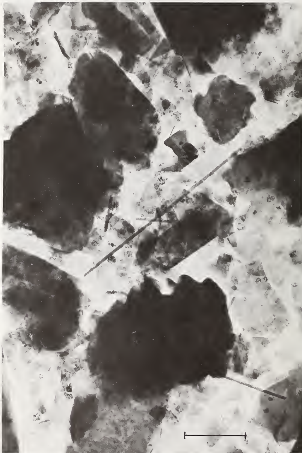
Figure 7. Commercial talc product with a 1% addition of chrysotile asbestos. Bar is one micron.
