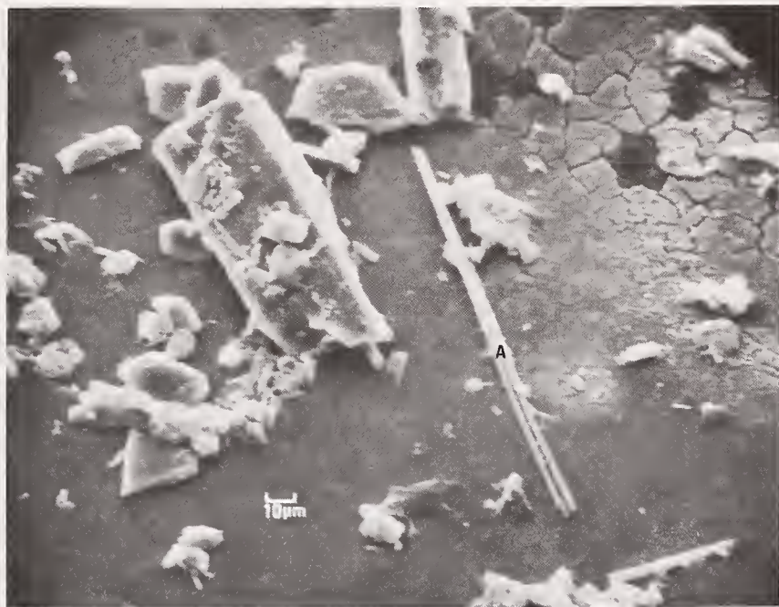
Figure 13. Platy talc, tremolite cleavage fragments, and a fibrous tremolite particle (A) (X 400).
