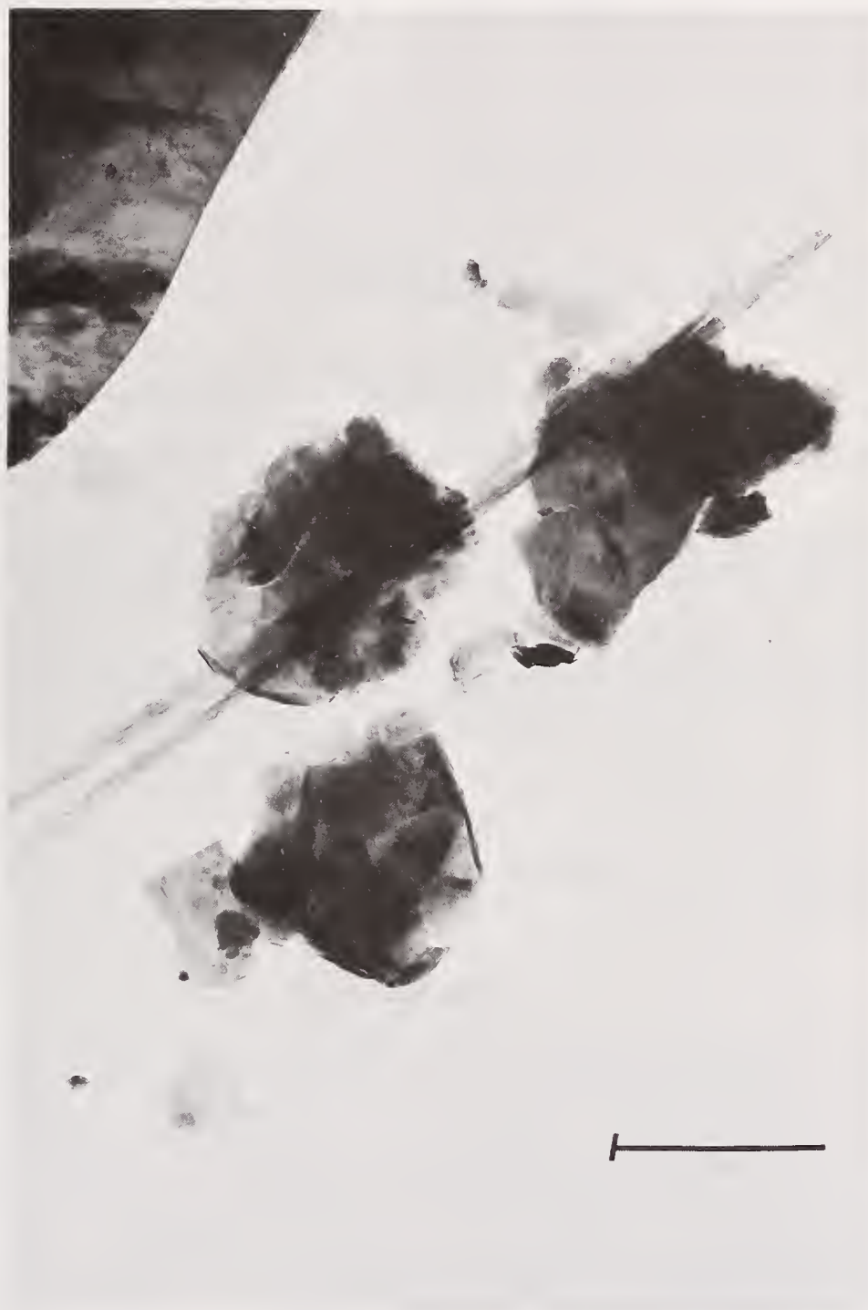
Figure 8. Commercial talc with naturally occurring co-deposits of chlorite and chrysotile asbestos. The asbestos is present at approximately the 1% concentration level. Bar is one micron.
