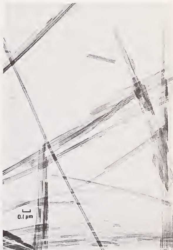
Figure 1. Chrysotile, showing individual fibrils, at two magnifications: X 18,000 (left) and X 35,000 (right). The hollow-tube structure is visible at the higher magnification. (TEM microphotographs.)
