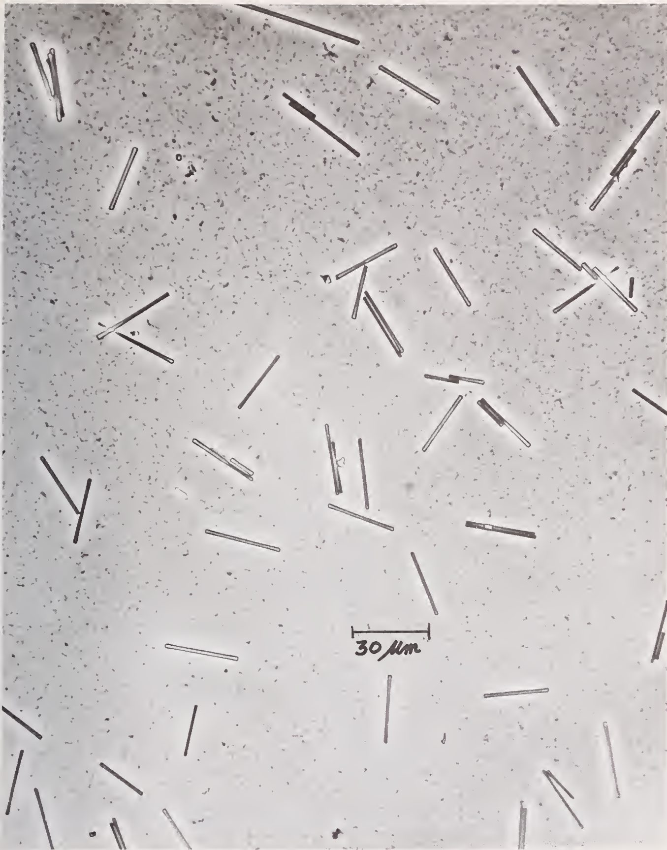
Figure 3. Glass fiber dispersion. Area near center of filter. Nominal dimensions of the fibers are 1.5 x 30 micrometers. Phase contrast.
