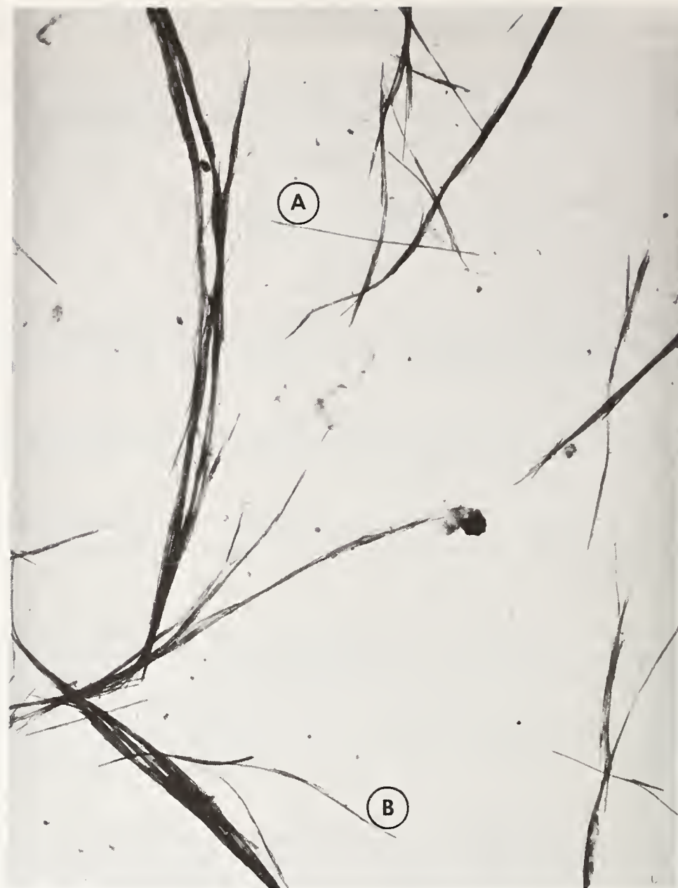
Figure 1. Ultrasonerated chrysotile suspension simulating size distribution of fibers shed from asbestos filters used for parenteral drugs — 3200 X.
