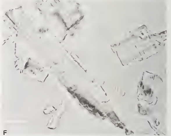
Figure 4. Light optical photomicrographs of tremolite asbestos and tremolite at three magnifications. Tremolite asbestos (left) at A , X 100; B , X 500; and C , X 950. Tremolite (right) at D , X 100; E , X 500; and F , X 950.
