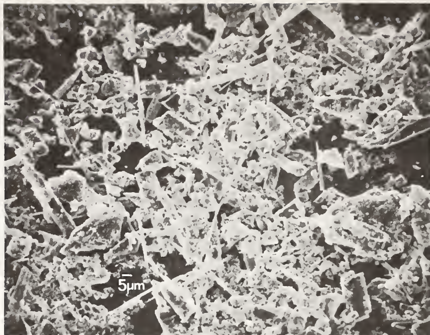
Figure 3. New York talc product used in the paint industry. Actual talc content is less than 40 percent. Majority of fibers are asbestos-tremolite, identified by TEM/SAED.
