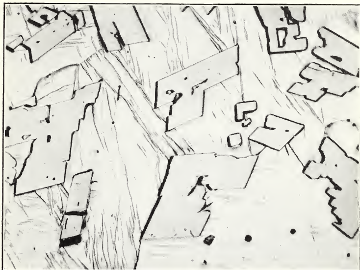
FIGURE 91.— Microstructure of zinc containing 1 per cent of iron, \times 100 The crystals are those of \text{FeZn}_7 (micrograph from The New Jersey Zinc Co.). Etching reagent: 100 ml water, 20 g chromic acid, 1.5 sodium sulphate.
