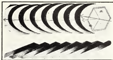
FIGURE 15.—Representation of the block movement along basal planes in a zinc single crystal
