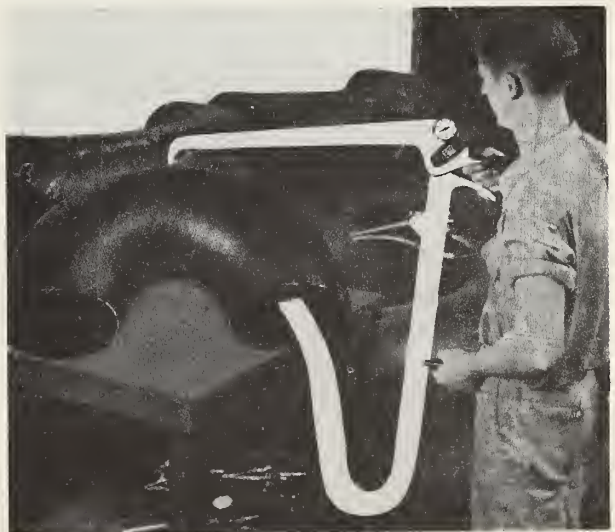
FIGURE 23. Combined joint caliper and dial gage to measure the wall thickness of elbow tubes.
