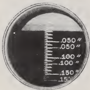
FIGURE 119. The two scales as reflected in the eyepiece when measuring glass approximately 18 mils thick.
