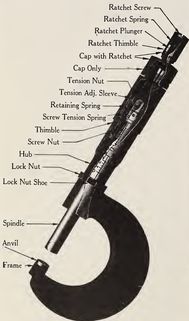
FIGURE 12. Micrometer caliper.
