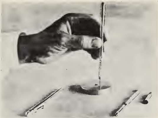
FIGURE 86. BSA/Tinsley pencil thickness gage.
