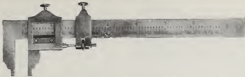
FIGURE 10. Slide caliper with vernier attachment.
