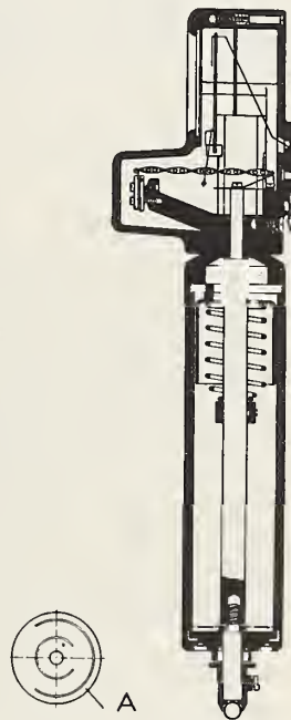
FIGURE 34. Lever magnification of movement.
