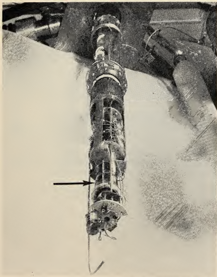
\text{He}^3 - \text{He}^4 dilution refrigerator produces temperatures below 0.1 K. Refrigeration is produced in a chamber inside a coil (arrow) used to measure the temperature. Suspended from the chamber are two devices to be tested—a Josephson-junction thermometer on the disc and a heat exchanger to the left. In use the refrigerator is surrounded by a vacuum space and several thermal shields.
