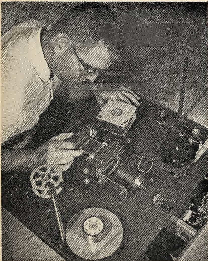
This microfilm rapid reader-copier, designed and built by the Bureau for the National Library of Medicine, is an example of services provided to other government agencies by the NBS Center for Computer Sciences and Technology.
