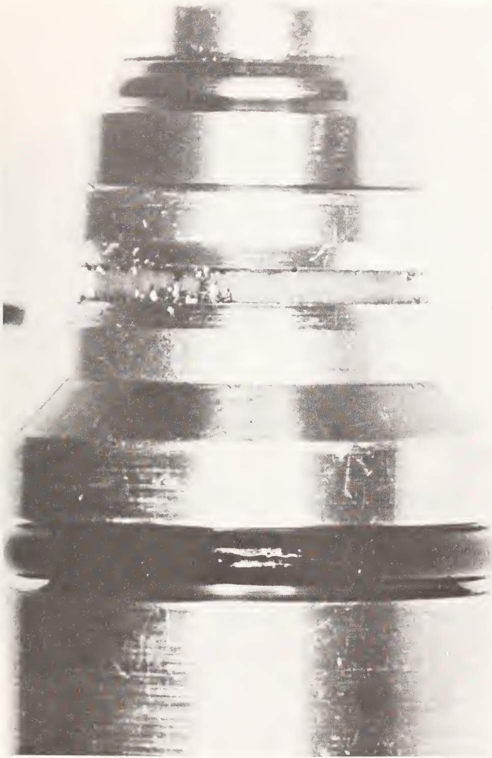
FIGURE 8: DEBRIS FROM FAILURE ILLUSTRATED IN FIGURE 7
