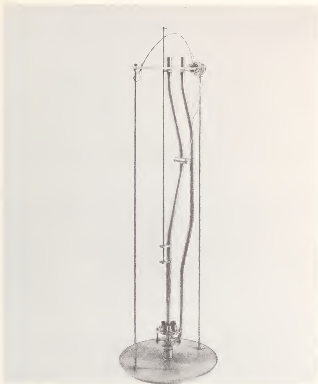
Figure 1. Isotopic neutron source holder and rabbit assembly.
