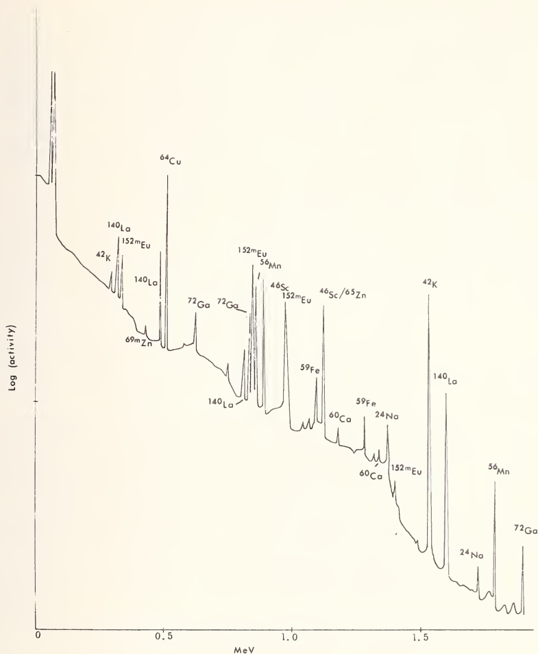
Figure 2. Ge(Li) spectrum of W-1 after ^{24}\text{Na} separation.
