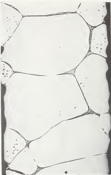
FIGURE 9: MICROGRAPHS OF SECTIONED COMPONENTS OF TEST (B, IRIIDIUM AND D ALLOY) AND REFERENCE (A, IRIIDIUM AND C, ALLOY) THERMOCOUPLES AGED AT 1850°C FOR 28 HOURS. THE MAGNIFICATION WAS 80X. FURTHER DESCRIPTION IS IN THE TEXT, 2.7.2. THERMOCOUPLE SYSTEM: IRIIDIUM-40% RHODIUM VERSUS IRIIDIUM.
