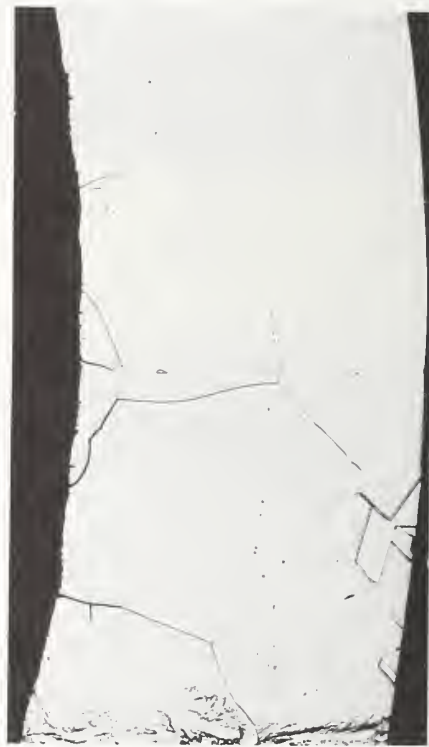
FIGURE 17: MICROGRAPHS OF SECTIONED ALLOY COMPONENT OF A TEST THERMOCOUPLE AGED AT 1500°C AND AT A GRADIENT OF 1475°C/CM FOR 60 HOURS. WIRE DIAMETER WAS 0.51 MM; THE MAGNIFICATION WAS 90X. PHOTOGRAPH A SHOWS A SECTION TAKEN 1.0 CM FROM THE JUNCTION; B, 0.5 CM FROM THE JUNCTION; AND C, 0.05 CM FROM THE JUNCTION. FURTHER DESCRIPTION IS IN THE TEXT, 3.7.2. THERMOCOUPLE SYSTEM: PLATINUM-13% RHODIUM VERSUS PLATINUM.
