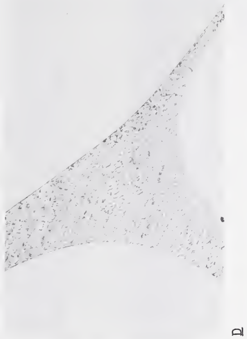
FIGURE 8: MICROGRAPHS OF SECTIONED IRIIDIUM-40% RHODIUM COMPONENT OF A TEST THERMOCOUPLE AGED AT 1700°C FOR 359 HOURS. PHOTOGRAPHS A, B, AND C WERE TAKEN WITH A MAGNIFICATION OF 100X; D, AN ENLARGEMENT OF A GRAIN-BOUNDARY PHASE FROM B, AT 1200X. FURTHER DESCRIPTION IS IN THE TEXT, 2.7.2. THERMOCOUPLE SYSTEM: IRIIDIUM-40% RHODIUM VERSUS IRIIDIUM.
