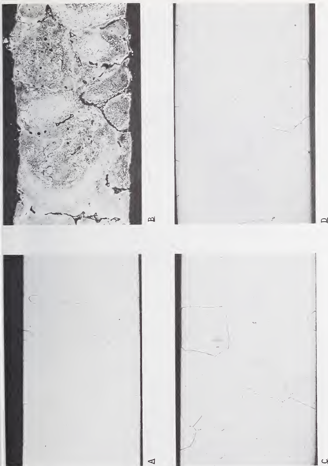
FIGURE 10: MICROGRAPHS OF SECTIONED COMPONENTS OF TEST THERMOCOUPLES UNHEATED (A, ALLOY AND C, IRIIDIUM) AND AGED AT 2000°C FOR 8 HOURS (B, ALLOY AND D, IRIIDIUM). THE MAGNIFICATION WAS 80X. FURTHER DESCRIPTION IS IN THE TEXT, 2.7.2. THERMOCOUPLE SYSTEM: IRIIDIUM-40% RHODIUM VERSUS IRIIDIUM.
