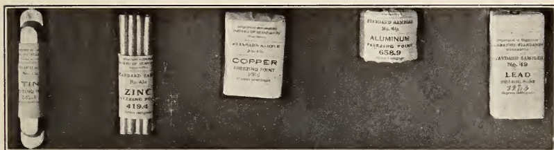
FIG. 29.— Standards for temperature fixed points (Freezing points)
