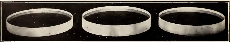
FIG. 27.—Standard of planeness (Quartz flats)
