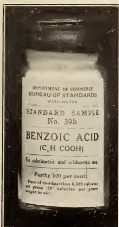
FIG. 2.—Standard for acidity measurement
