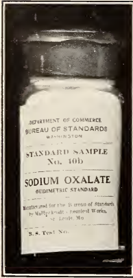
FIG. 24.—Oxidimetric standard (Pure sodium oxalate, \text{Na}_2\text{C}_2\text{O}_4 )
