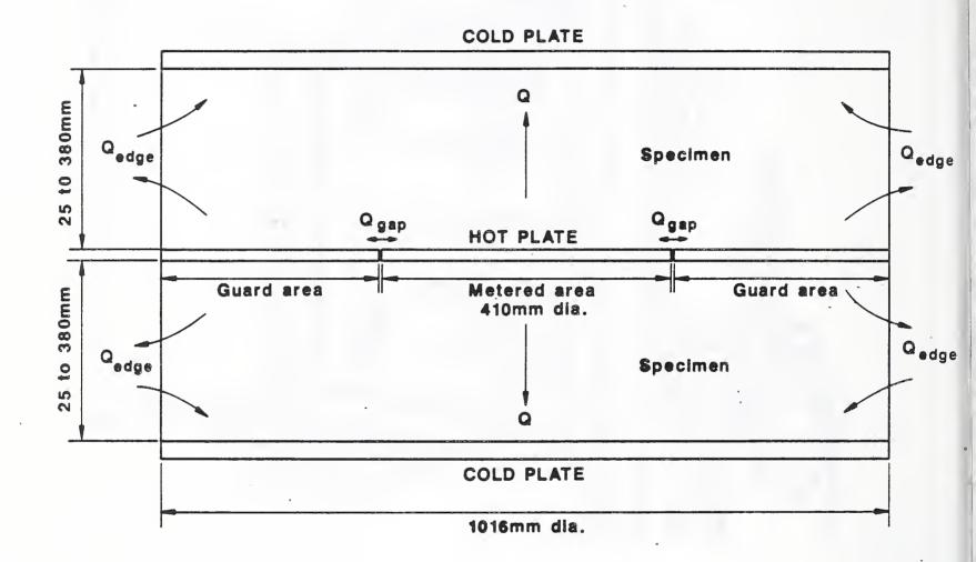
Fig. 2. Principle of measurement for the NBS 1-metre Guarded Hot Plate in a two-sided mode of operation.
