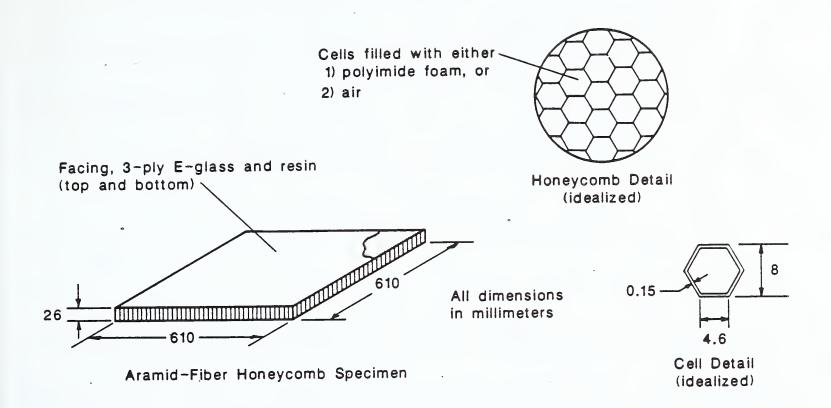
Fig. 3. a) Honeycomb structure of the aramid-fiber honeycomb specimens.
