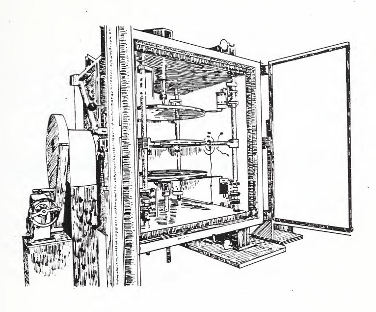
Fig. 1. The NBS 1-metre Guarded Hot Plate.
