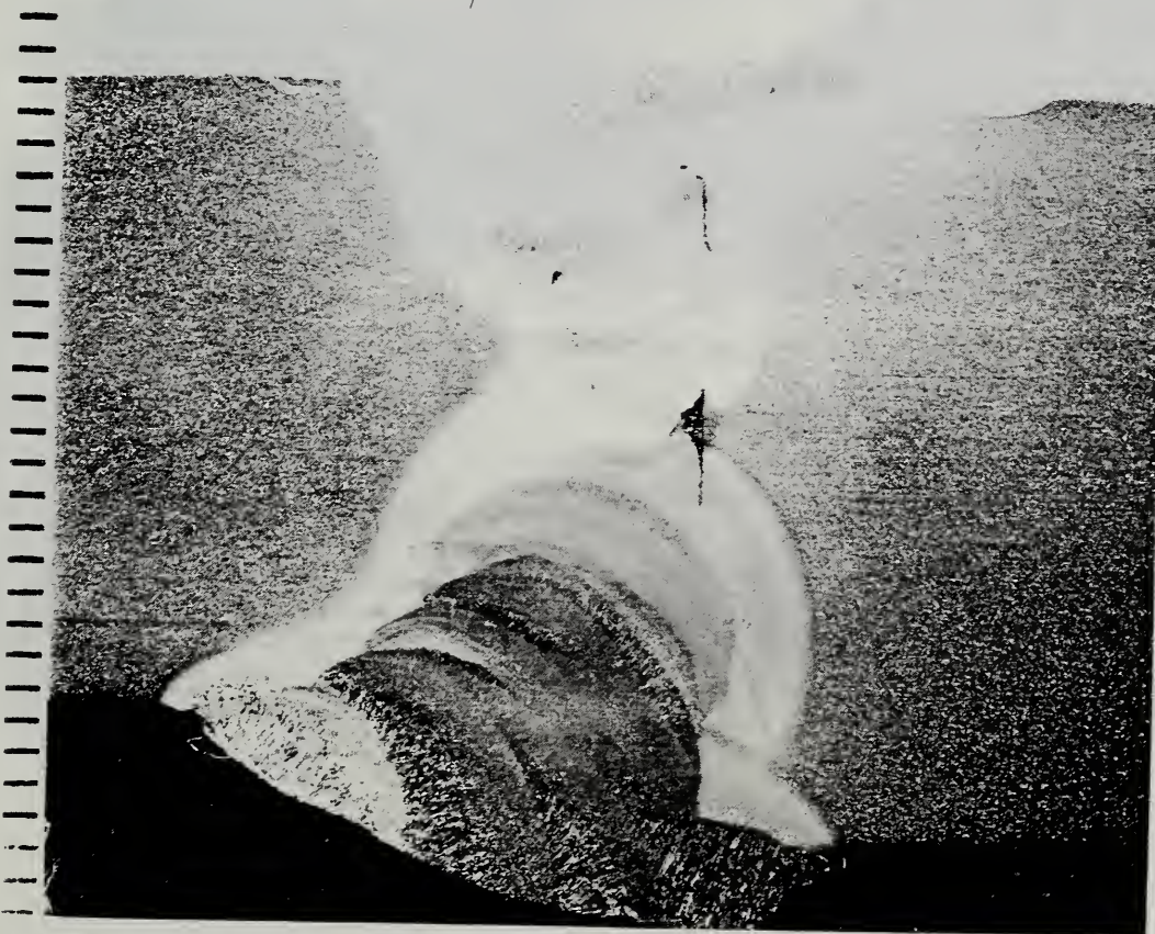
Figure 5.4.10 Cross section showing the weld in specimen NBS 4-F1 (x 4)
