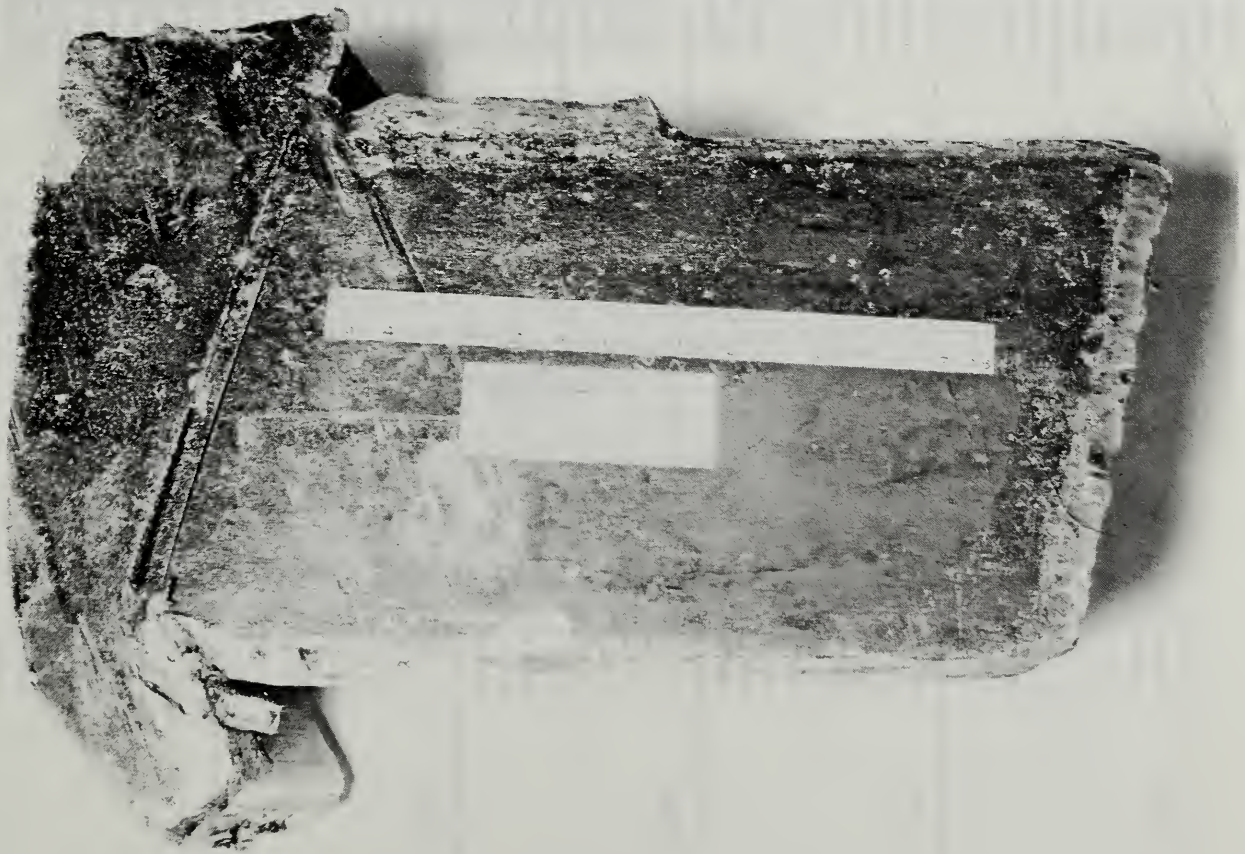
Figure 5.4.13 NBS specimen 33A, weld block/wedge sample from debris
