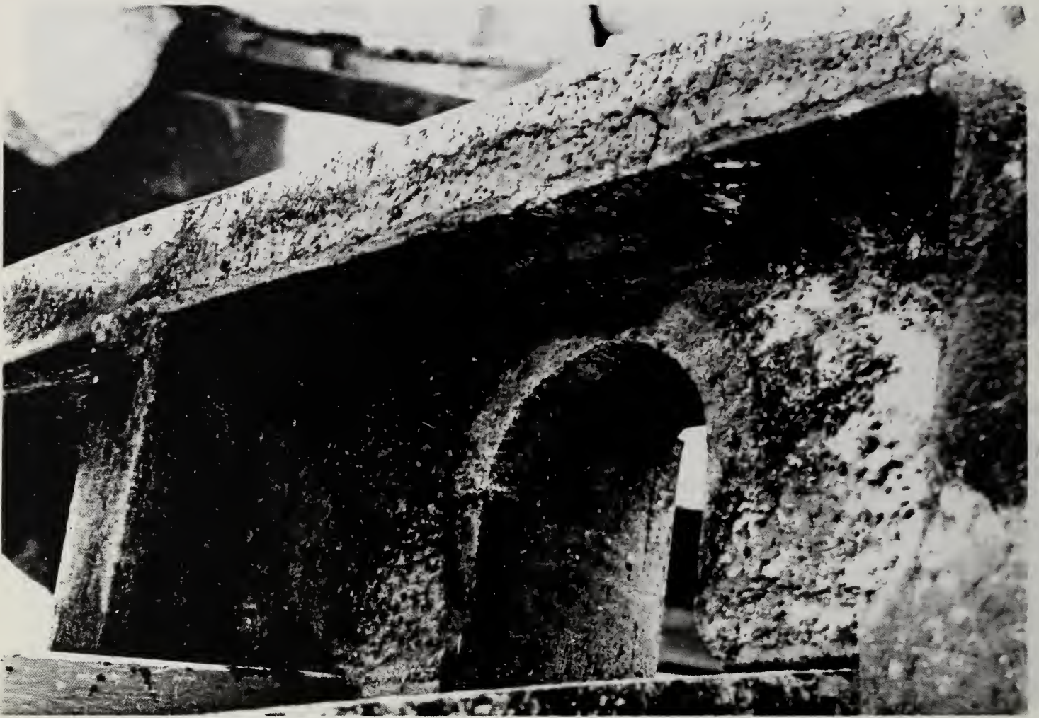
Figure 4.4.33 Typical indentation in underside of lifting angle
