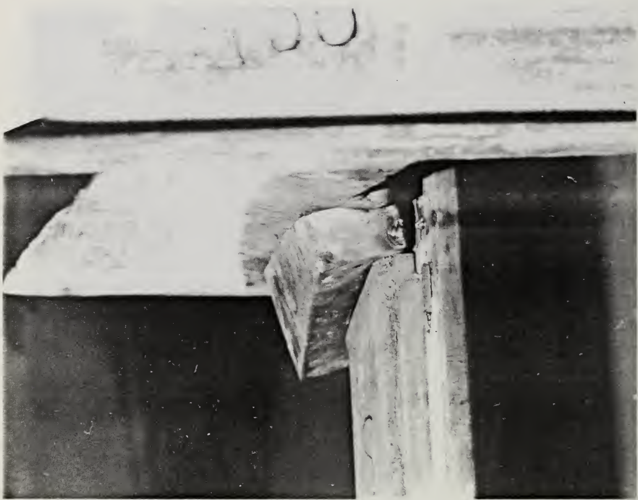
Figure 5.5.12 Deformation of shearhead channel in test of shearhead
