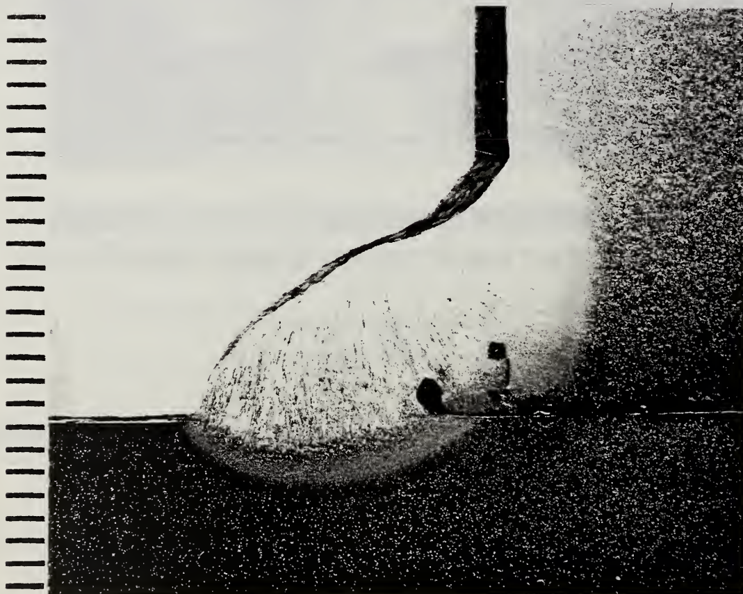
Figure 5.4.4 Cross section showing weld in sample NBS-3A-3 (x 4)
