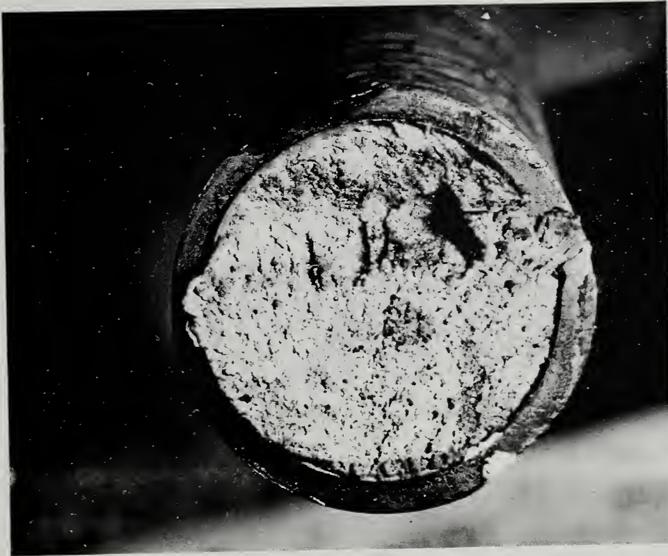
Figure 5.5.5 Fracture surface of jack rod, sample NBS 11-2 (x 1)
