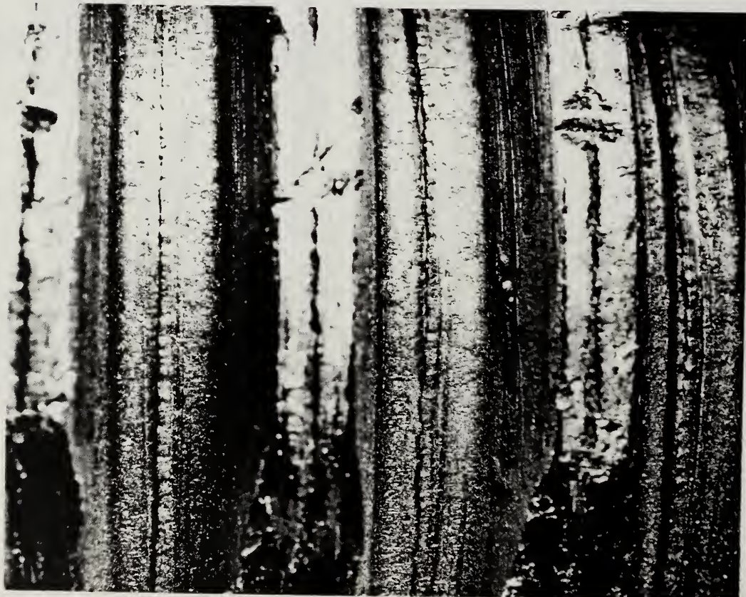
Figure 5.5.4 Jack rod on tension side showing lap seam from thread rolling operation (x 3)
