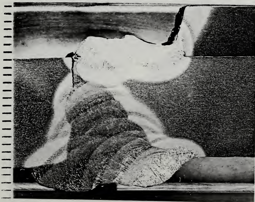
Figure 5.4.6 Cross section showing weld in specimen NBS 8-T1 (x 4)
