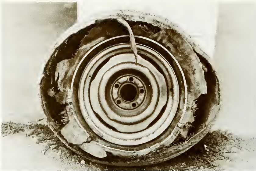
FATAL HIGH SPEED FAILURE OF STANDARD GRADE PASSENGER TIRE (ALABAMA STATE POLICE – 1974)
