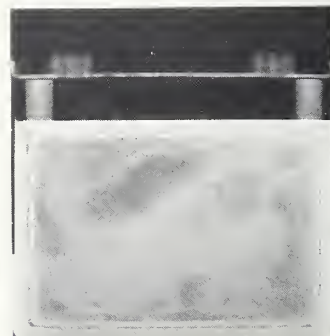
Figure 7. Neutron radiograph of a lithium-iodine battery with 102-percent depletion.
