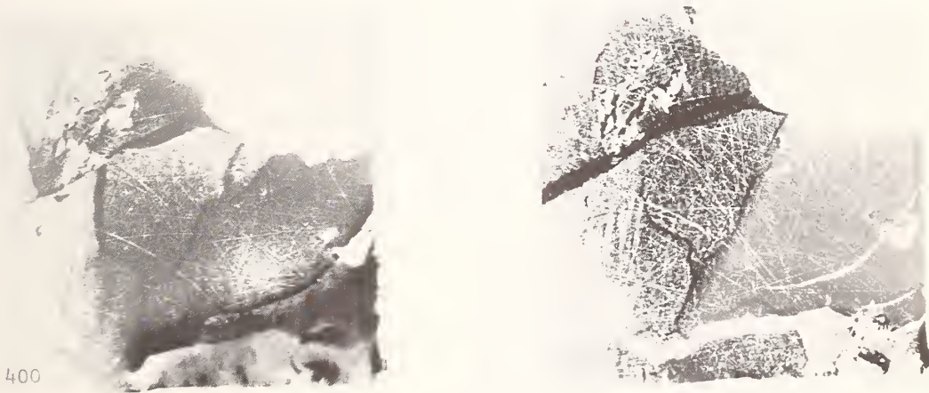
Figure 5. X-ray topographs of a mechanically polished (100) ALQLOY surface.
