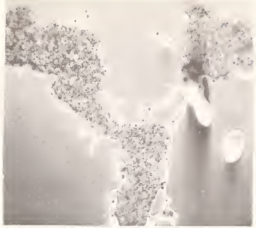
Figure 14. Detail of damage to bias sputtered silver shown in Figure 13; 395 \text{ J/cm}^2 (700X).
