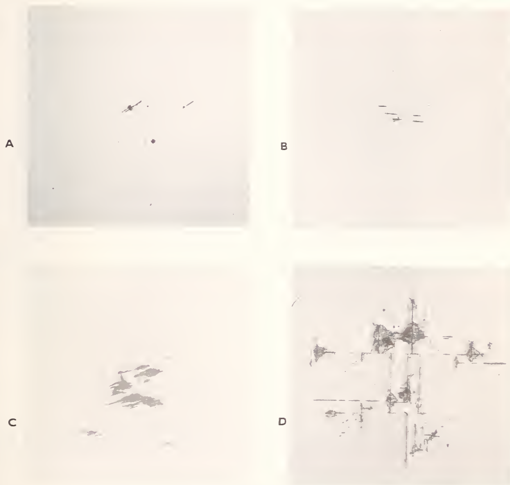
Figure 3. Typical exit damage sites. (a) at 3.0 joules/cm 2 , Harshaw, 50x (b) at 3.8 joules/cm 2 , Harshaw, 50x (c) at 3.8 joules/cm 2 , Harshaw, 50x (d) at 2.5 joules/cm 2 , Harshaw, 50x.
