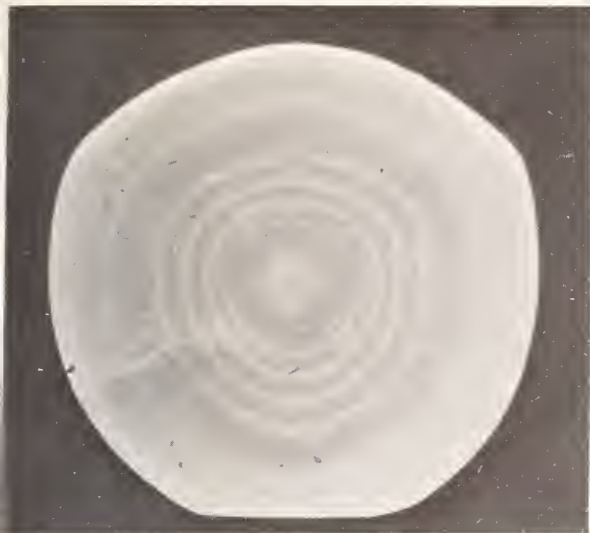
Figure 7. \text{LiNbO}_3 crystal used in Figures 5 and 6, photographed after etching in HF. Crystal diameter: 5/8".
