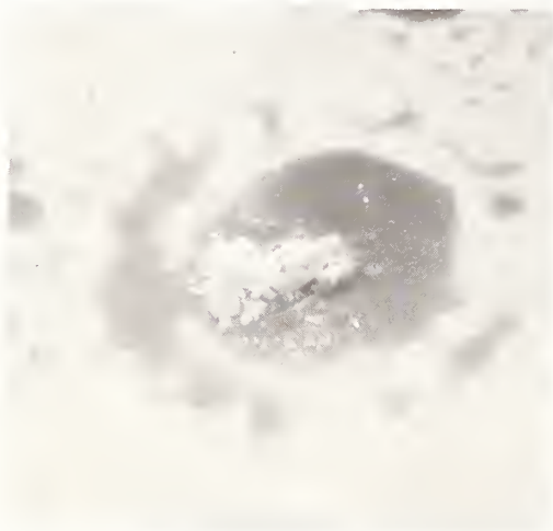
Figure 17. Detail of smaller damage spot on un-overcoated silver film shown in Figure 15; 229 J/cm 2 (2100X).
