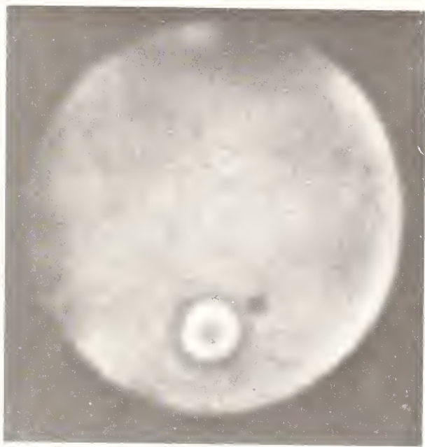
Figure 12. Thermally stimulated exoelectron image of a polished LiF single crystal after exposure to 45 min of 50 kV, 15 mA X-rays and subsequently to a single 2.3 J 50-nsec pulse from a Nd glass laser. There was no observable surface damage.
