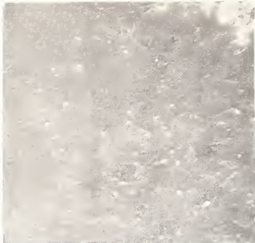
Figure 8. Detail of most heavily damaged part of Figure 6, showing partial removal of coating by blister formation and bursting, 233 \text{ J/cm}^2 (1000X).
