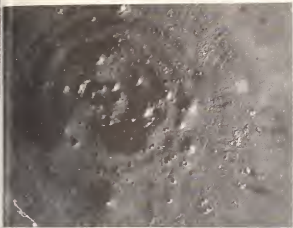
Figure 10. Optical micrograph taken using Nomarski lens. Note interference rings within the damage. Photo shows 1.1 mm width.
