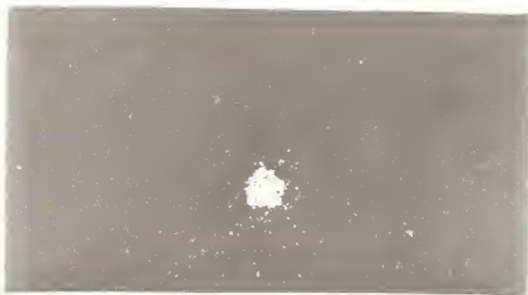
Figure 4b. Single crystal germanium, 20 \Omega \times \text{cm} , n-type. Fifty shots at 7.5 \text{ J/cm}^2 in 75 nsec (damage obtained once only). Magnification is \times 100 .
