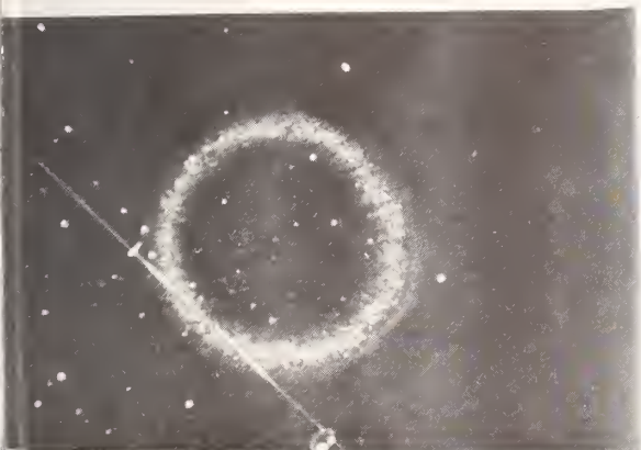
Figure 2a. Single crystal germanium, 20\ \Omega \times \text{cm} , n-type. One shot at 17\ \text{J}/\text{cm}^2 in 75 nsec. Magnification is x 50.
