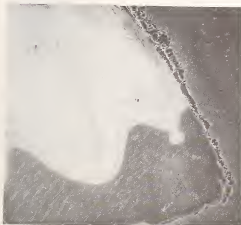
Figure 21. Damage to aged (4 months) uncoated gold film on beryllium copper substrate; R = 0.990 , 347 \text{ J/cm}^2 (80X).
