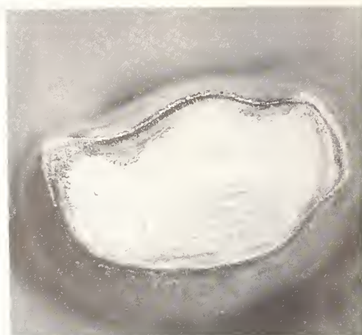
Figure 3. Vacuum evaporated \text{ThF}_4/\text{Ag} coating on Berylco 25 substrate aged 4 months in ambient atmosphere. R = 0.992 ( \lambda = 5 \mu\text{m} ). CO laser, 278 \text{J}/\text{cm}^2 (80X).
