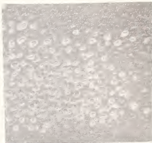
Figure 6. Damage to beryllium copper mirror coated with evaporated ThF 4 /Ag, exposed to ambient air for 4 months prior to CO laser testing; R = 0.991, 416 J/cm 2 (80X).
