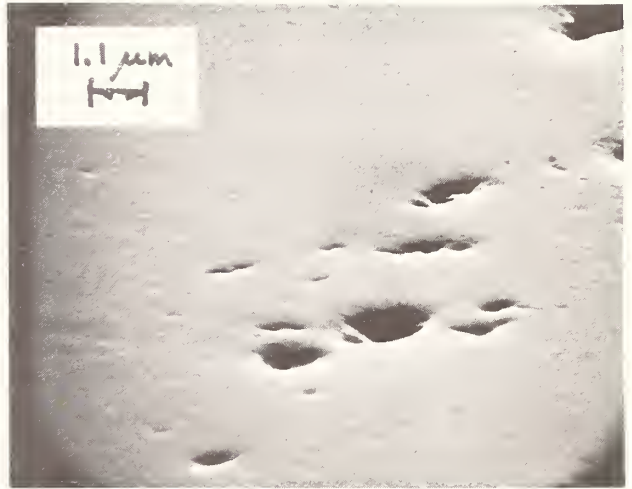
Figure 7. SEM photograph of defects of a group of holes on a single quarter-wave \text{MgF}_2 film.
