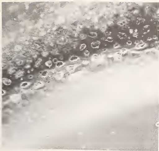
Figure 4. Detail of edge of damage area of Figure 3, 278 J/cm 2 (700X).
