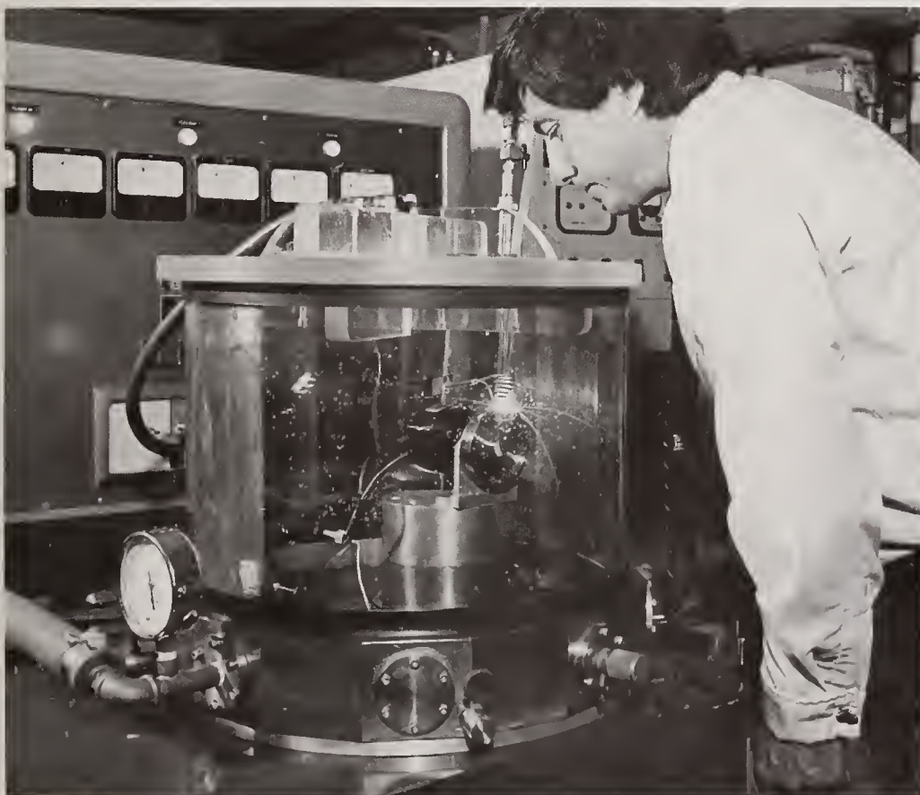
Melt Spinning Apparatus in the Metals Processing Laboratory
