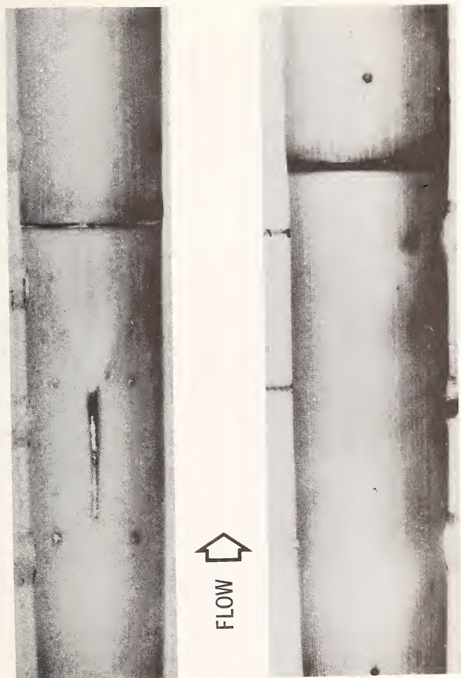
FIG. 3 ABLATION PATTERN IN TEFLON DUCT OBTAINED IN "LAMINAR" RUN
