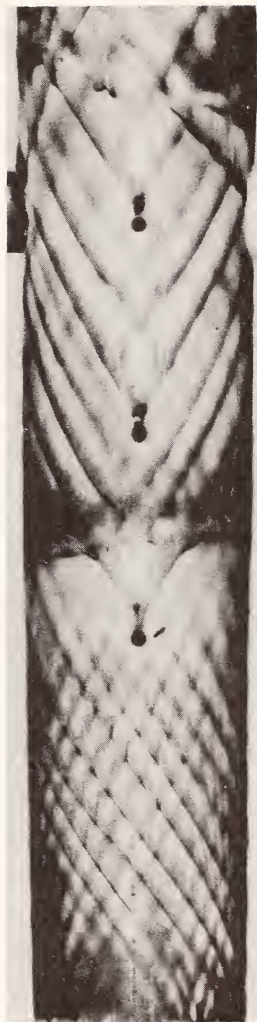
FIG. 5 CROSS - HATCHED STRIATION PATTERN
