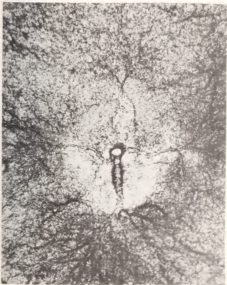
Figure 1. Photomicrograph of FEP Film After Puncture Has Occurred Using 25 Kev Protons at 10^{12} p/cm. 2 -sec. to 10^{16} p/cm. 2 (Magnified 100×)
