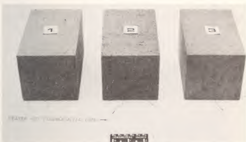
Figure 4.- Heat-shield samples used in the thermal conductivity study.
