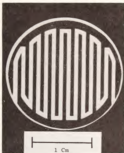
Fig. 1—Configuration of vapor deposited gold electrode.
