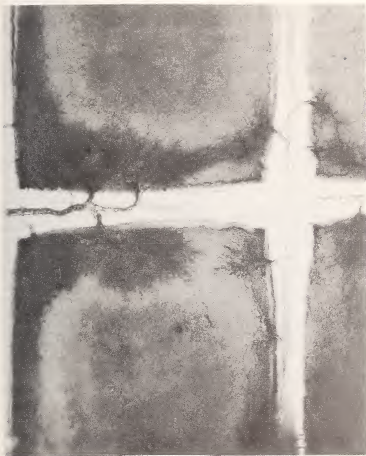
Figure 6. Photomicrograph of Silver Coated FEP After Irradiation With 30 Kev Electrons at 10^{12} p/cm. 2 -sec. to 10^{15} p/cm. 2 Showing Extensive Veining Beneath Charge Shadowed Regions
