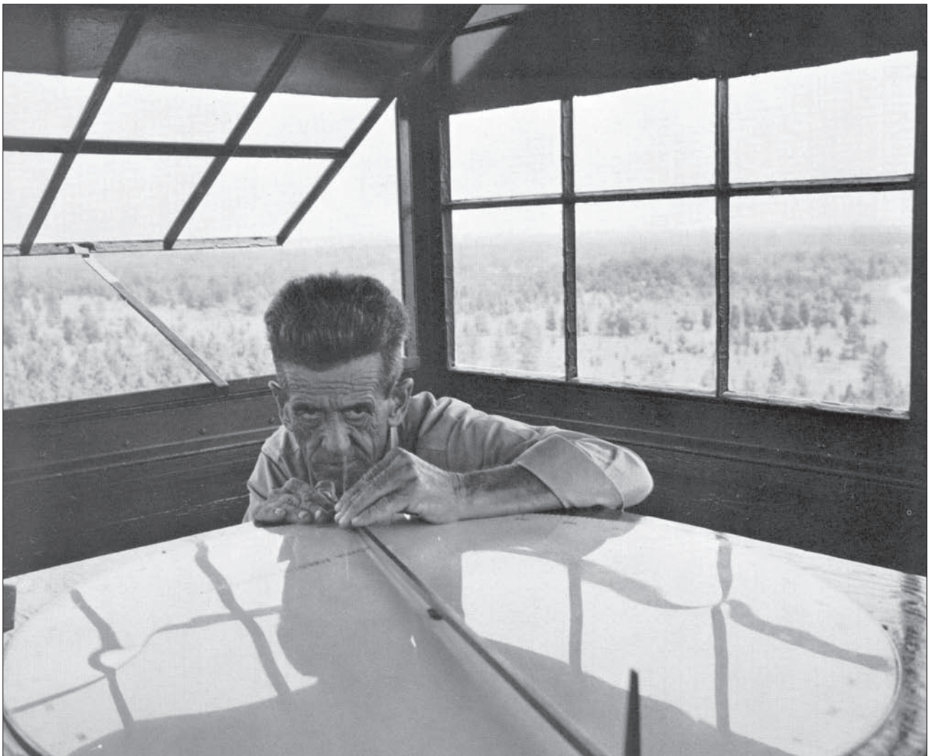
Tower man in a lookout using an alidade to determine the location of a wildfire. (Photograph by Elemore Morgan)
