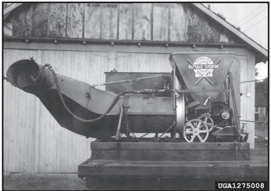
Figure F-1. This insecticide mist blower, designed and constructed in 1946 by Quincy Forestry Department, Massachusetts, was used to spray trees in residential areas.
