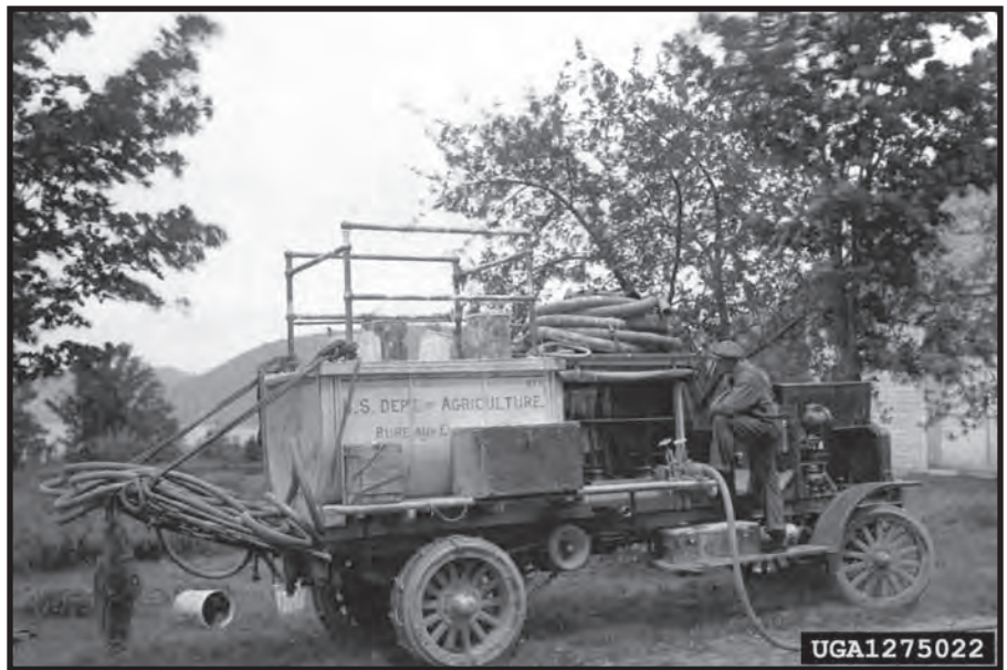
Figure K-1. A sprayer unit mounted on a Model A Ford truck was used for gypsy moth control.
