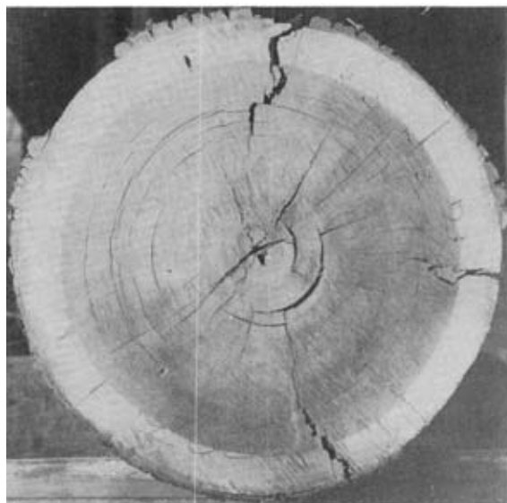
Figure 2.--Splits and shake in this sweetgum log were caused by alternate freezing and thawing.
