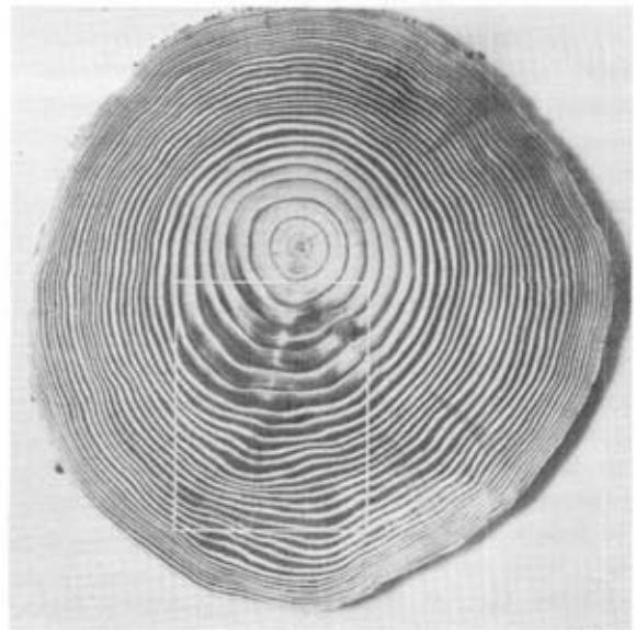
Figure 6.--Compression wood in a southern pine log.
