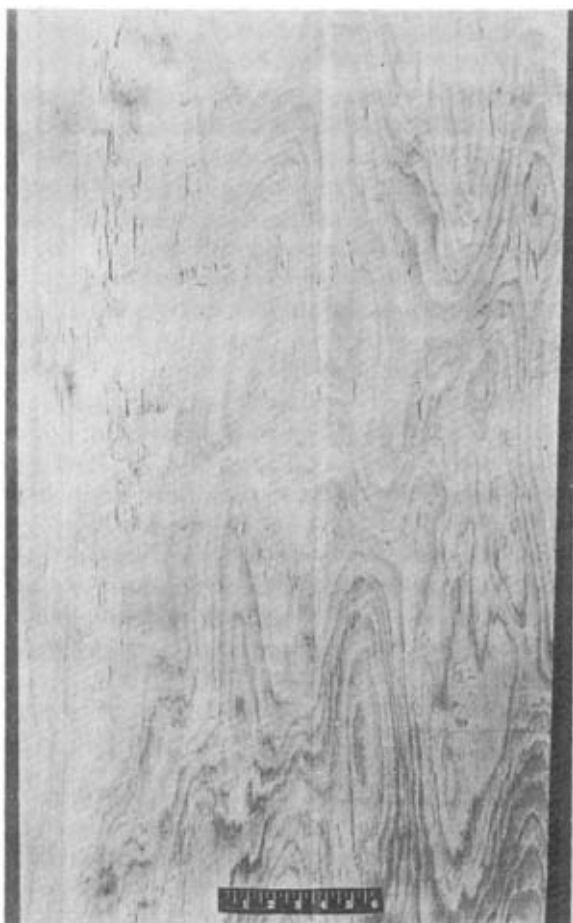
Figure 1 .--"Shelling" or shattering of redwood veneer that was rotary-cut from a "sinker" log. The scale is in inches.
