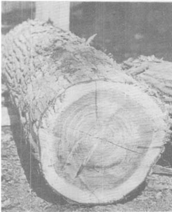
Figure 5.--Tension wood in a cottonwood log. (M 75160)
