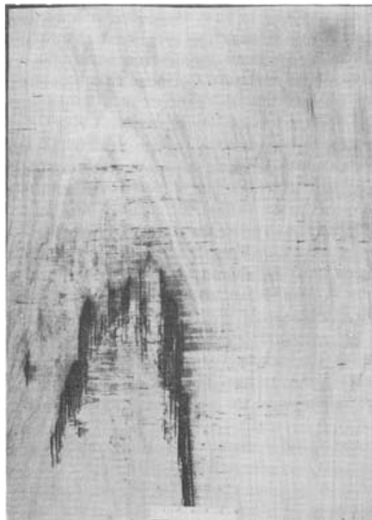
Figure 4.--Gum in a sheet of rotary-cut Brazil nut veneer. (M 136 441)
