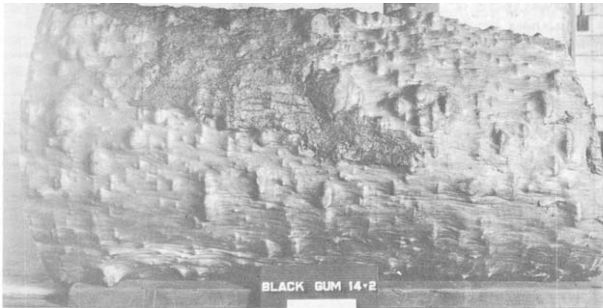
Figure 9.--A bolt of black gum with many burls on the surface, Veneer cut from this bolt is shown in figure 10. (M 91476 F)
