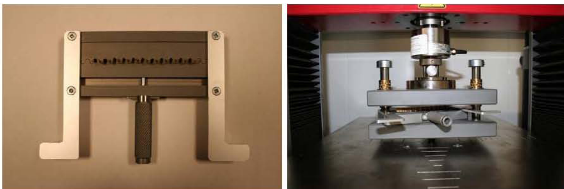
Figure 2: CCT-holder and compression tester.
