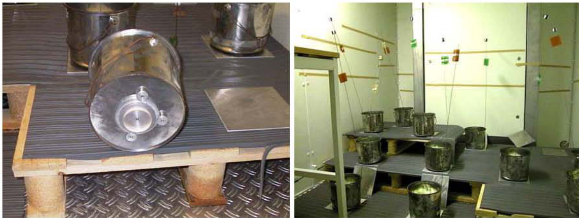
Figure 1: The setup for the "lead bucket method", based on RCT for creep studies of fluting paper. To the right several rigs placed in a climate chamber.
