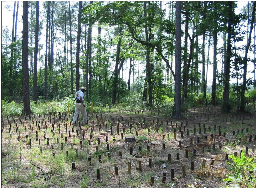
Figure 4. Ground-contact stake testing is conducted for years as part of evaluating a wood preservative.
