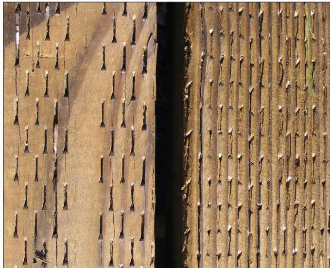
Figure 7. Examples of the appearance of lumber that has been incised prior to pressure treatment to increase the depth and uniformity of preservative penetration.
