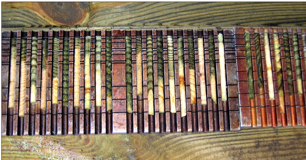
Figure 5. Each pressure-treated charge (cylinder load) of wood is inspected by removing increment cores from 20 or more pieces. Preservative penetration is measured on the cores, and then the portion corresponding to the assay zone is removed for chemical analysis of preservative retention.
