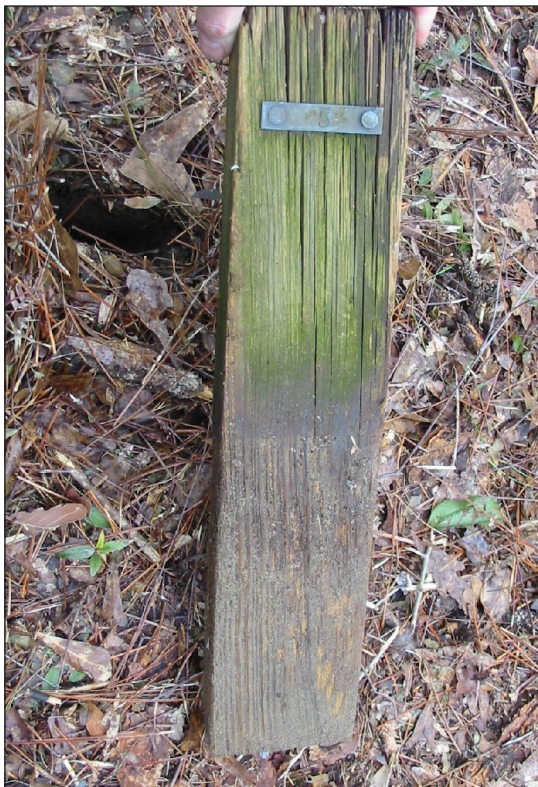
Figure 27. This pressure-treated 2 by 4 lumber specimen has remained in good condition for more than 60 years of exposure at the USDA Forest Service, Forest Products Laboratory test site in southern Mississippi.
