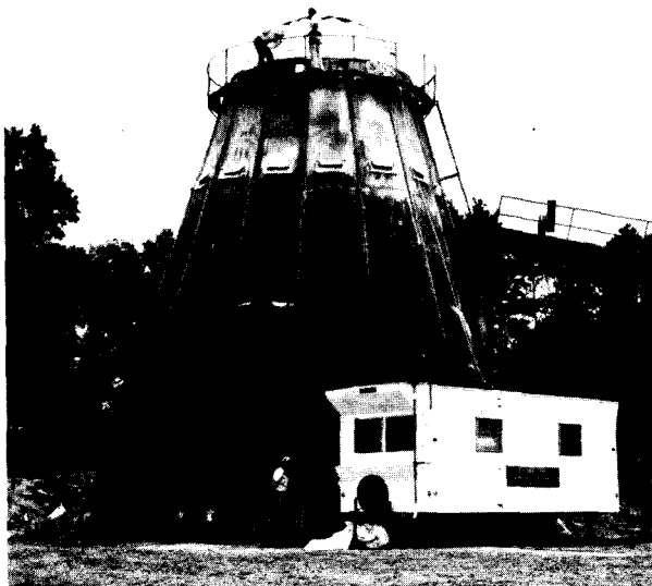
Figure 5.--A teepee burner was converted into an experimental combustion chamber. Emission monitors were installed at the teepee outlet.
