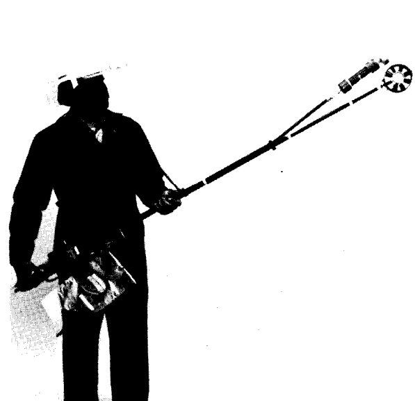
Figure 4.--Portable sampler for monitoring emissions from burning forest fuels.
