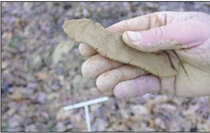
Forming a ribbon indicates silt loam or clay texture soil that should allow a site to hold water.
