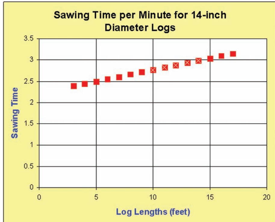
Figure 11. —SOLVE's regression routine for sawing times per log estimates the sawing time data that lie outside of the range that contains sawing times entered by the user (indicated by an X marked on the data points that lie between log lengths of 10 and 14 feet). The trend in this chart is linear and the data points show little variation. This indicates a strong relationship between log length and sawing time.
