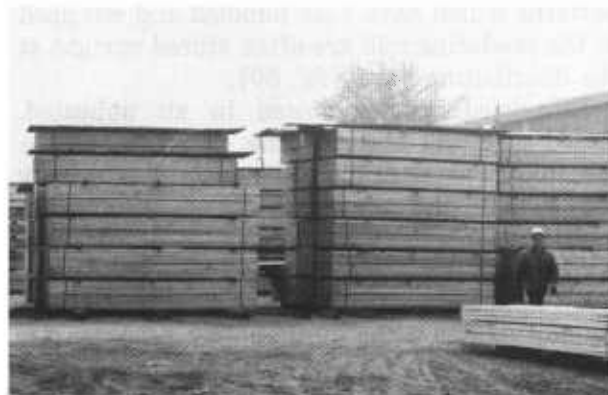
Figure 45.—Outdoor storage of dry, finished softwood lumber. Note the use of pile roofs to provide some protection from rain and sun.
