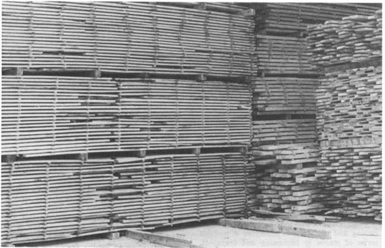
Figure 1. —Green lumber will lose moisture when it is stored, and should be stickered as shown here for controlled, even drying.
