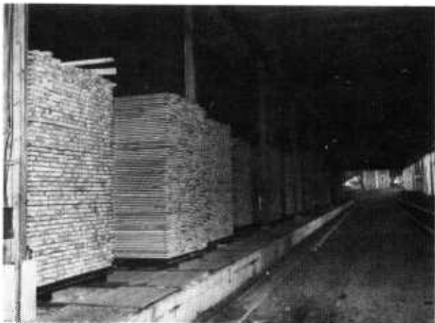
Figure 55.—Kiln-dried lumber stored in a cooling shed on kiln trucks. The doors at the two ends of the transfer track are usually closed.
