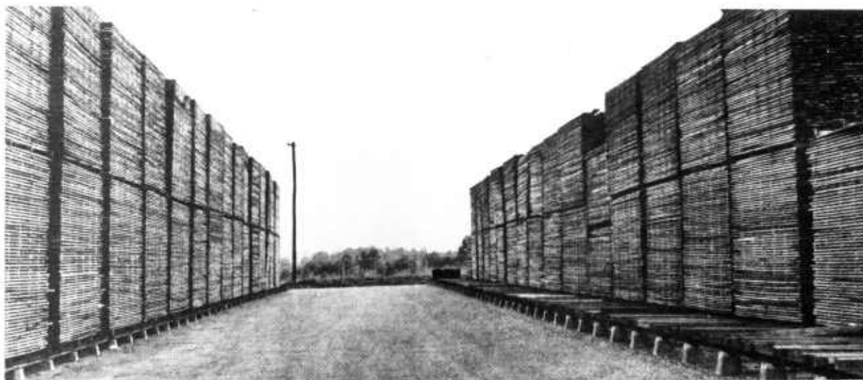
Figure 20.—Stickered unit packages of hardwood lumber piled on permanent foundations in a “line-type” forklift yard.
