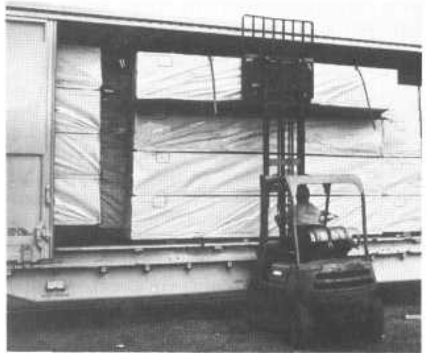
Figure 4.—A forkloder places a wrapped package of lumber in a wide-door boxcar. The paper wrap will temporarily protect the lumber when stored outdoors at its destination.
