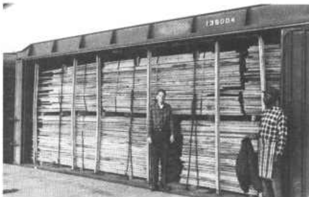
Figure 37.—Wide-door box car designed for fork truck handling of packages of kiln-dried lumber. Note corner irons and ratchet-type load binders.
