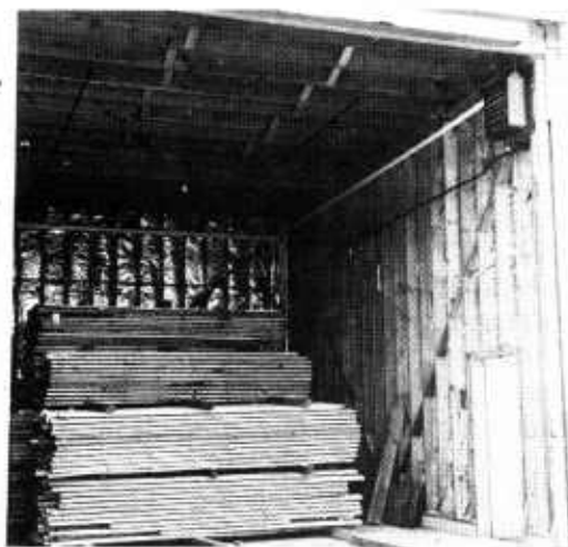
Figure 56.—Kiln-dried lumber stored in a heated shed at a furniture factory. A. Sliding doors provide access for lift trucks with packages of lumber. B. Kiln-dried lumber on stickers stored in an insulated, heated storage shed. Note the unit heater in the shed's upper right-hand corner.
