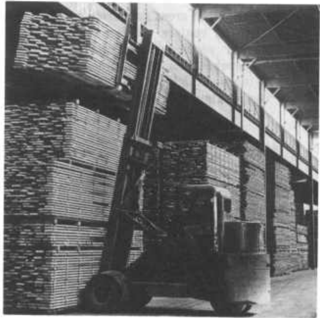
Figure 29.—Stickered lumber undergoing conditioning in a closed, unheated cooling shed.
