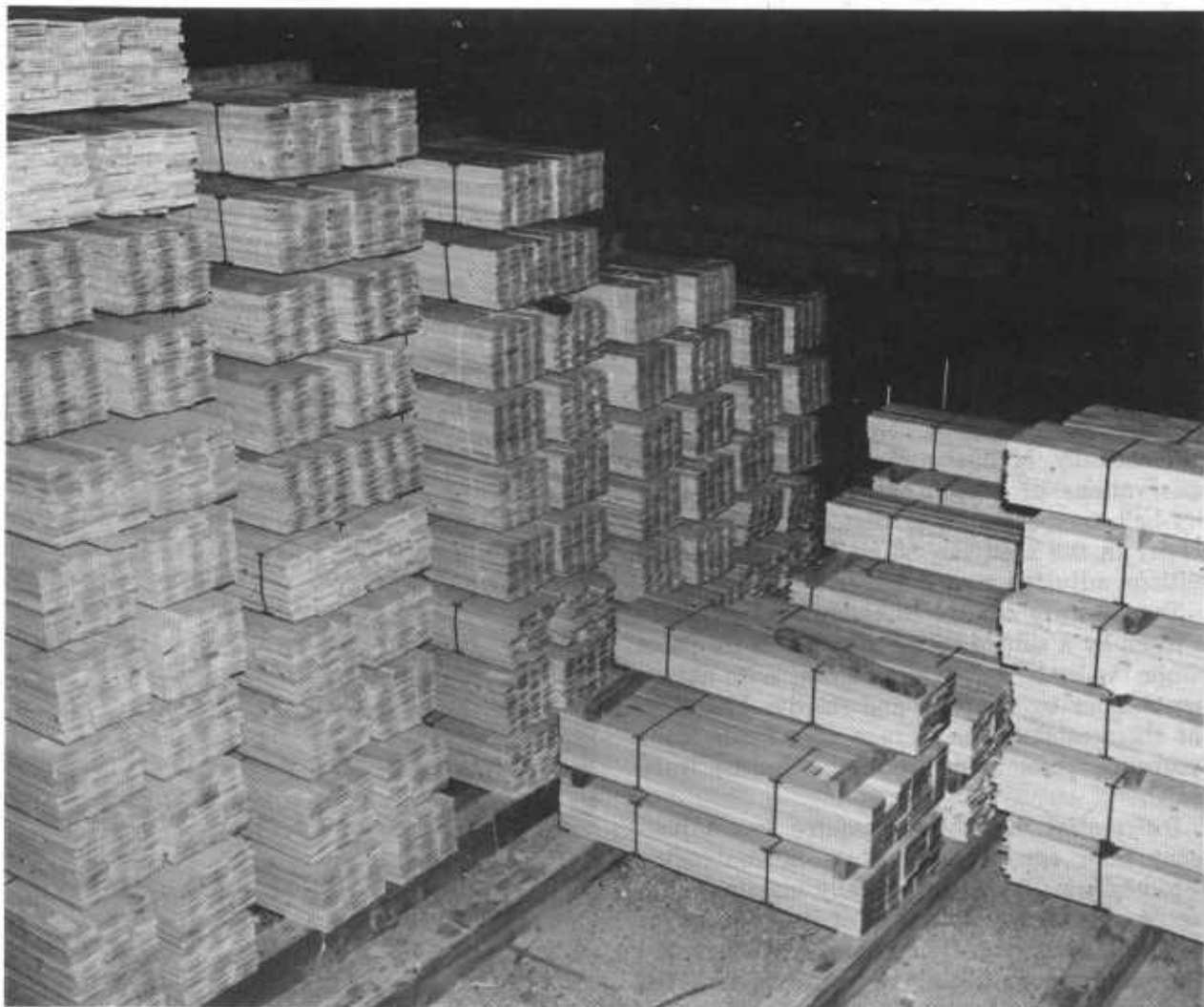
Figure 26.—Dry, finished softwood lumber stored as unit packages in a large, unheated shed at a western sawmill. High, close-spaced stacks are made possible by use of an overhead crane.
