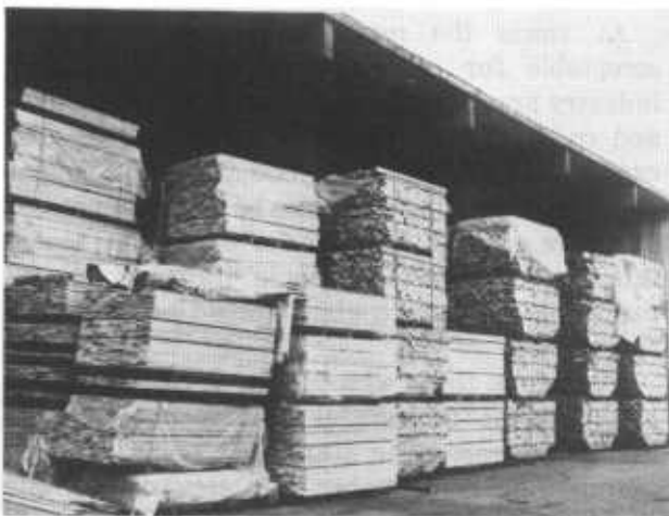
Figure 2. —Pallet packages of lumber stored in an open shed. Some packages have been unitized with iron bands (center). Others are clad in plastic film for additional protection.
