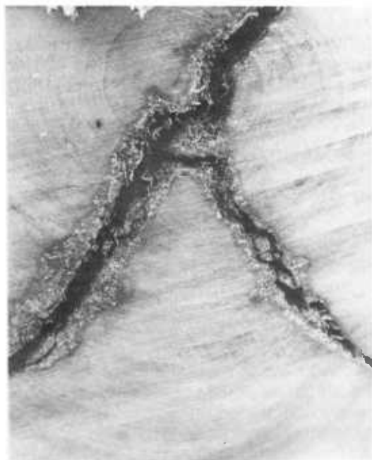
Figure 7-19. White ring rot ( Poria albipellucida ) along the checked surface of a redwood log.
