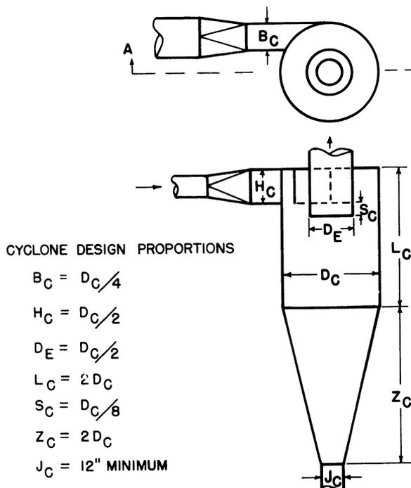
FIGURE 4-26.—Relative dimensions for a small-diameter design cyclone.
