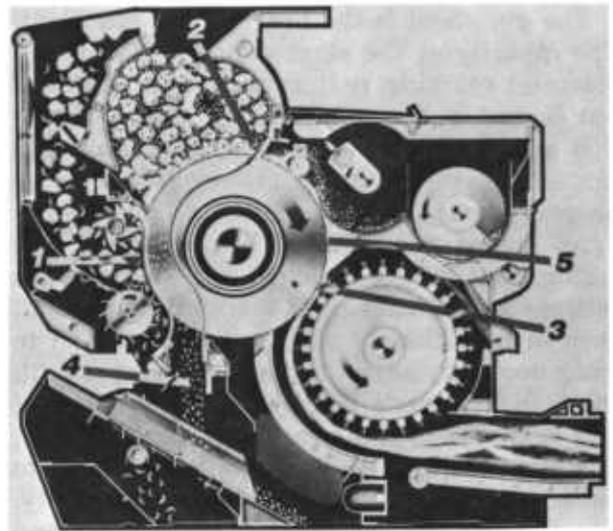
**FIGURE 3-33.**—Important settings and adjustments for Murray 142-18 brush gin. 1, Saw projection through huller rib,  $\frac{1}{2}$ ". 2, Ginning point to point of rib, 2". 3, Brush to saw, depth of sawteeth. 4, Foot of huller rib to ginning rib, 3". 5, Mote bar to saw,  $\frac{3}{8}$ ". Saw speed, 545 revolutions per minute.
