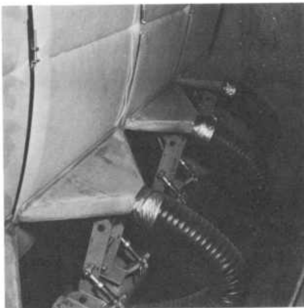
FIGURE 4-40.—Vacuum nozzles doffing filter drum covered with nonwoven polyester media.
