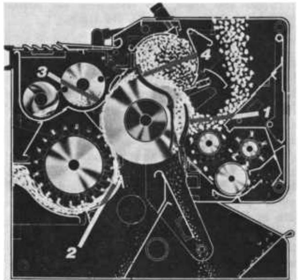
FIGURE 3-30.—Important settings and adjustments for Continental/Moss-Gordin Comet 141 saw-brush gin. 1, Saw projection through huller rib,  $\frac{3}{8}$ ". 2, Gravity mote board to brush,  $1\frac{1}{2}$ ". 3, Overhead mote board to saw,  $\frac{3}{8}$ ". 4, Ginning point to point of rib, 2". Saw speed, 700 revolutions per minute (r/min). Brush speed, 1,850 r/min.
