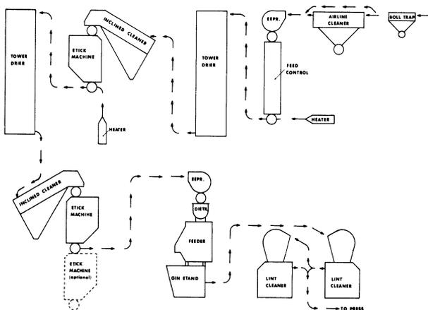
FIGURE 6-2.—Recommended gin machinery arrangements for stripped cotton.
