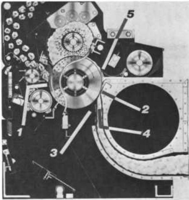
FIGURE 3-34.—Important settings and adjustments for Lummus Imperial 128 saw airblast gin. 1, Saw projection through huller rib,  $\frac{1}{2}$ " to  $\frac{3}{8}$ ". 2, Airblast nozzle to saw,  $\frac{1}{8}$ ". 3, Airblast mote board to saw,  $\frac{1}{4}$ ". 4, Airblast throat opening,  $1\frac{1}{8}$ ". 5, Overhead mote lip to saw,  $\frac{1}{8}$ ". Saw speed, 830 to 855 revolutions per minute. Airblast pressure, 16" to 19" of water.
