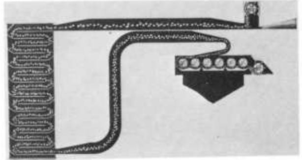
FIGURE 3-6.—Typical gin drying system. A fan and burner deliver heated air to the air-cotton pickup point, and a second fan is usually used to aid in conveying cotton through the system.
