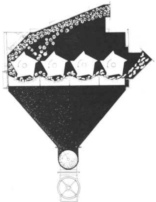
FIGURE 3-17.—Flow of cotton through an air-line cleaner.
