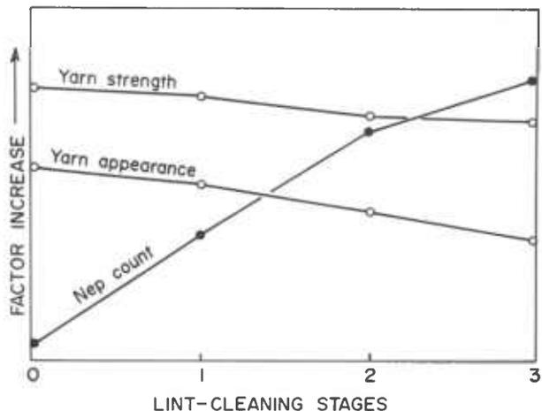
FIGURE 3-47.—Effect of saw lint cleaners on nep count, yarn strength, and appearance.
