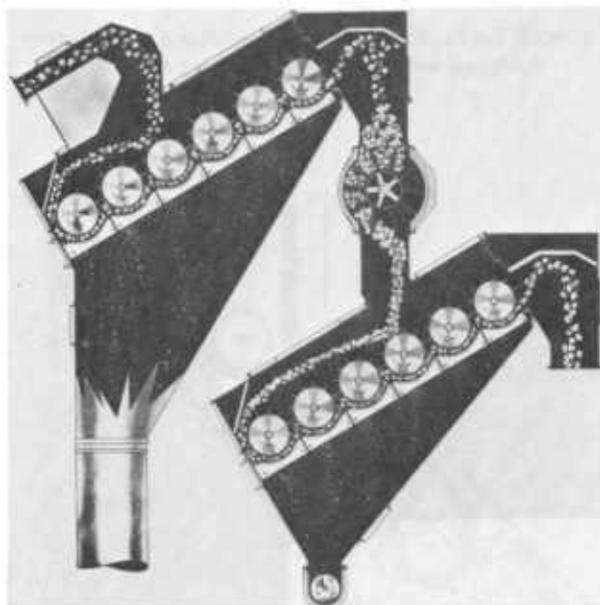
FIGURE 3-19.—Hot-air cleaner discharging into a gravity cleaner.
