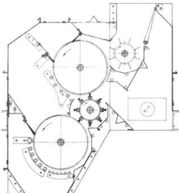
FIGURE 3-25.—Gravity-fed, two-saw stick machine with brush doffing cylinder.
