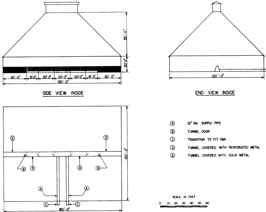
FIGURE 4-22.—Aeration layout of a Muskogee-type, or peak-loaded, storage.
