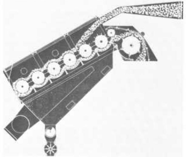
FIGURE 3-12.—Flow of cotton through an inclined cleaner.
