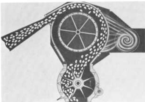
FIGURE 4-5.—Separator with revolving screen drum (Bush-Hog/Continental Gin).
