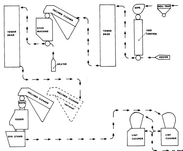
FIGURE 6-1.—Recommended gin machinery arrangements for machine-picked cotton.
