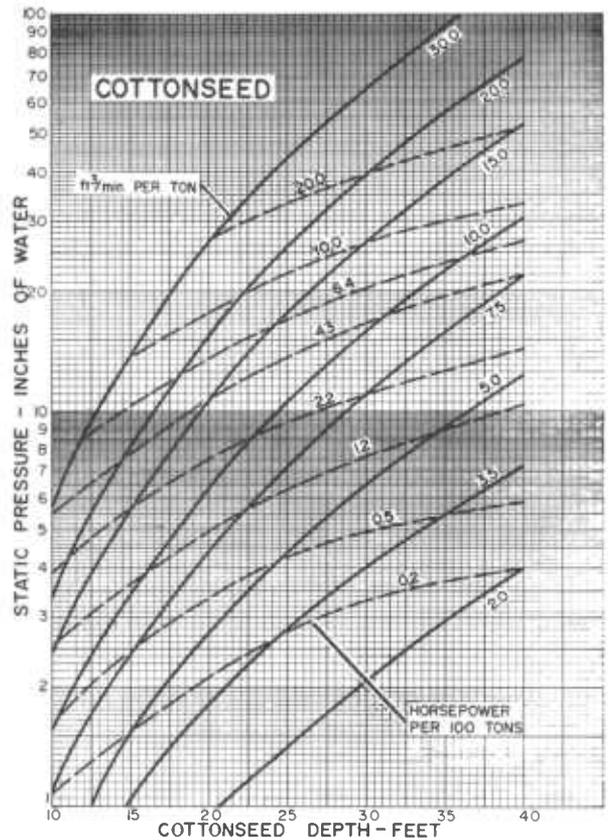
FIGURE 4-20.—Fan horsepower and static pressure requirements for aerating cottonseed at various airflow rates and at cottonseed depths from 10 to 40 feet.
