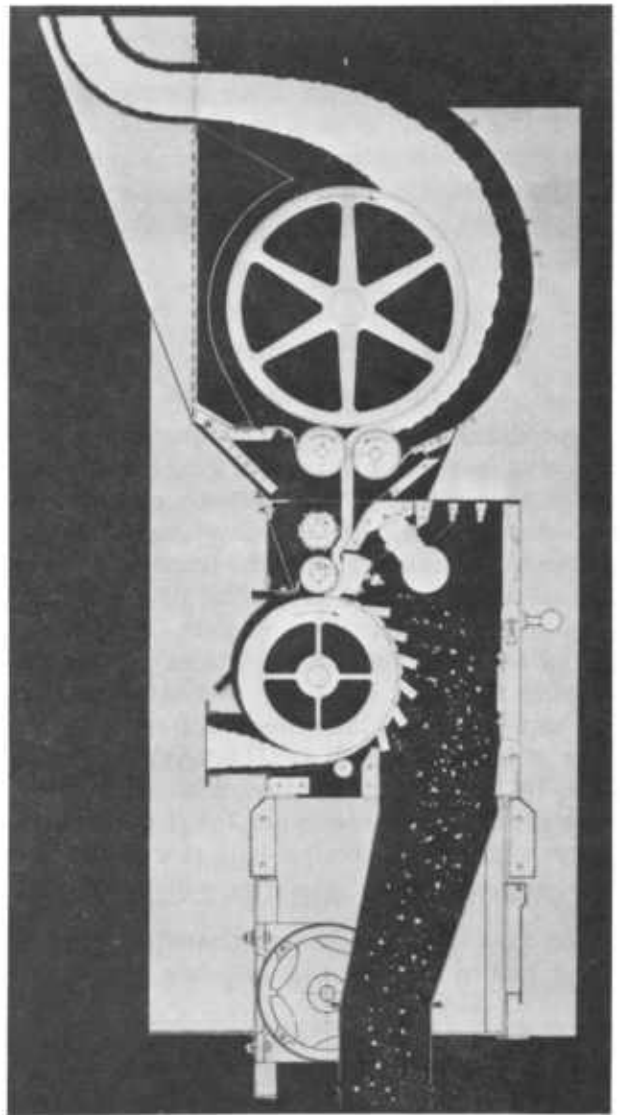
FIGURE 3-43.—Unit controlled-batt saw lint cleaner with air suction doffing (Lummus model 66 or 86 lint cleaner).
