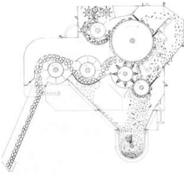
FIGURE 3-27.—High-capacity feeder with extracting and cleaning features.
