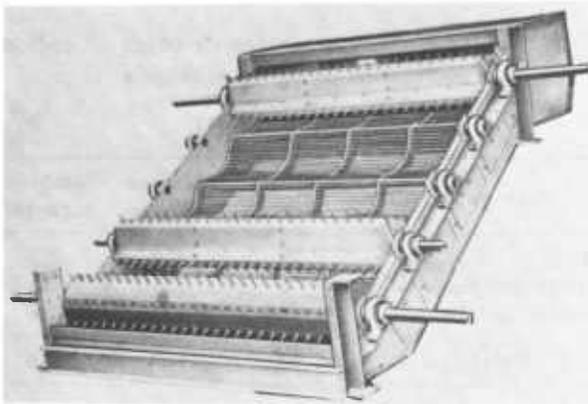
FIGURE 3-10.—Inclined cylinder cleaner equipped with grid-rod screen.
