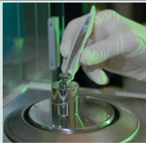
Specialists in the Engineering and Facilities Management Services unit calibrate scales like this one to ensure accuracy in all measurements.
