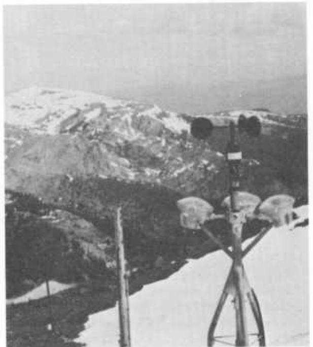
Figure 45.—The formation of rime on wind sensors (left). One solution is to heat the sensors with infrared lamps (right). (Photos by Judson)
