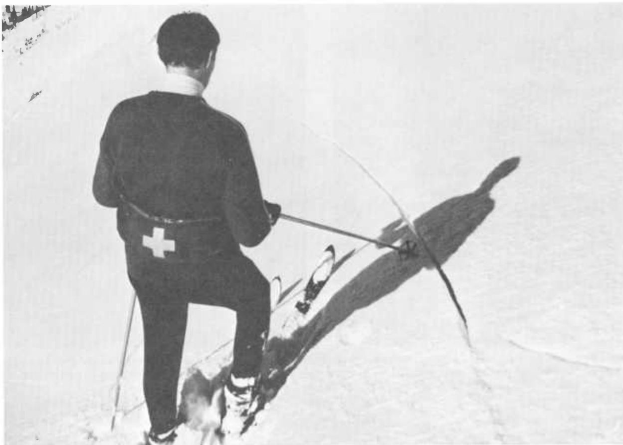
Figure 129.—Fracture propagation is direct evidence of instability. Fractures may propagate from the tester's skis or, in cases of extreme instability, around the periphery of the slab. (Photo by LaChapelle)
