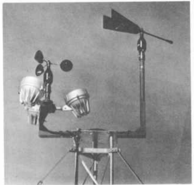
Figure 44.—Rotating-cup anemometer and wind vane. These instruments should be located on a high, isolated ridgecrest and set on a tower at least 3 m above the ridge.
