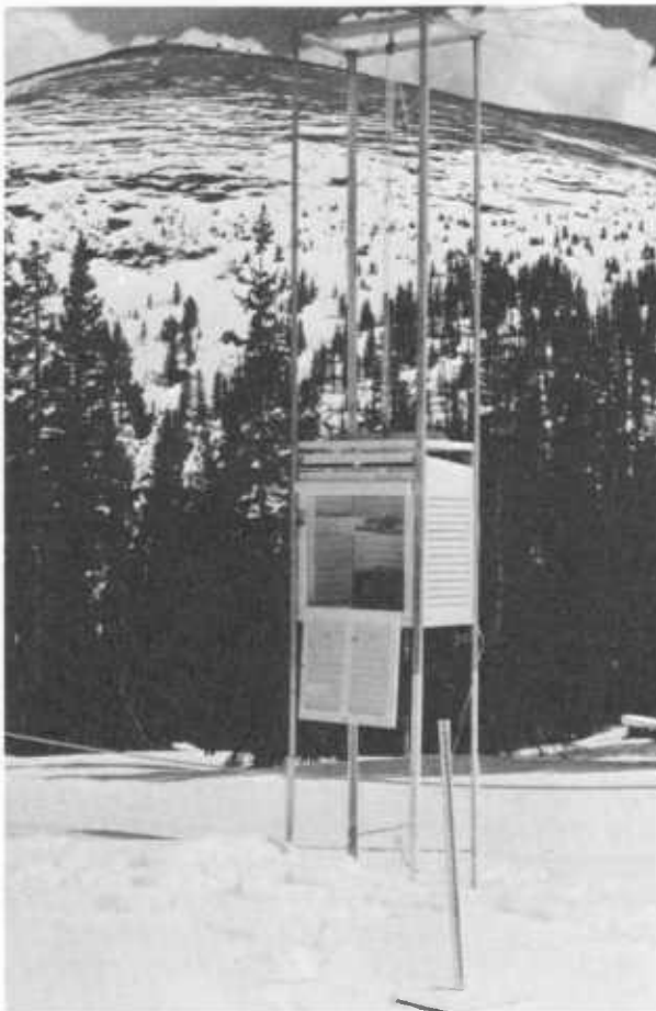
Figure 50.—Standard instrument shelter for housing thermometers and other meteorological instruments. The metal frame and pulley allow the shelter to be raised or lowered to keep it the proper height above the snow.
