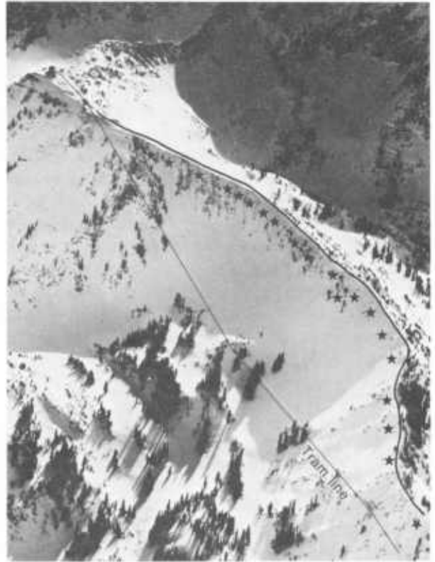
Figure 141.—Target areas along control routes at a Utah ski area. Explosives should normally be placed within the slab boundaries about halfway between the slab center and crown. If possible, the radius of influence should sweep into shaded pockets where structural weakness is likely to be most pronounced.
