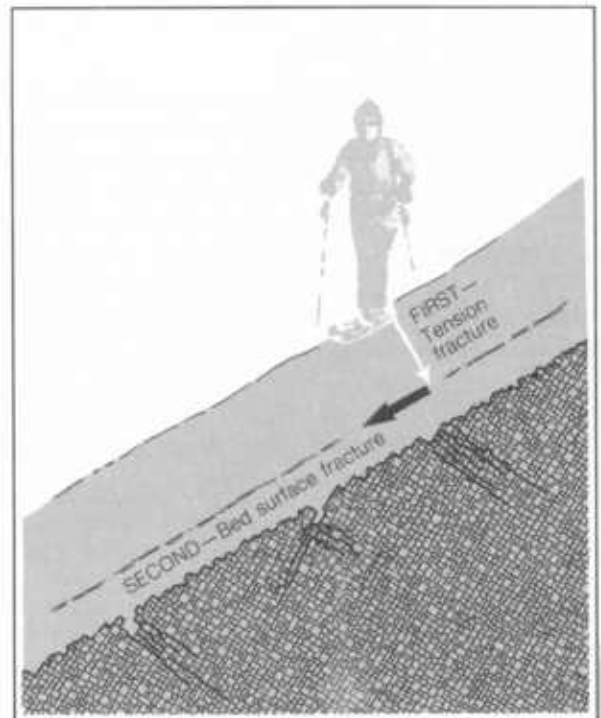
Figure 100.—Initial failure may occur as a tension crack. The opening of the tension crack would induce shear fracture at the bed surface.
