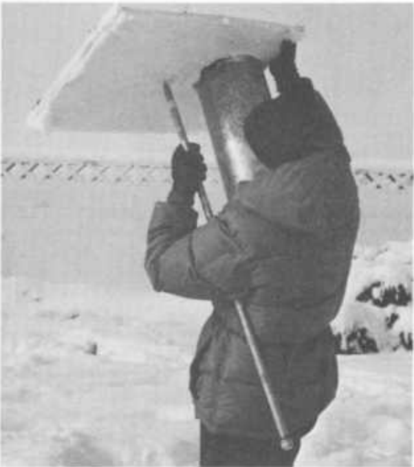
Figure 22.—Gathering and weighing a core sample of precipitation from a portable snowboard.
