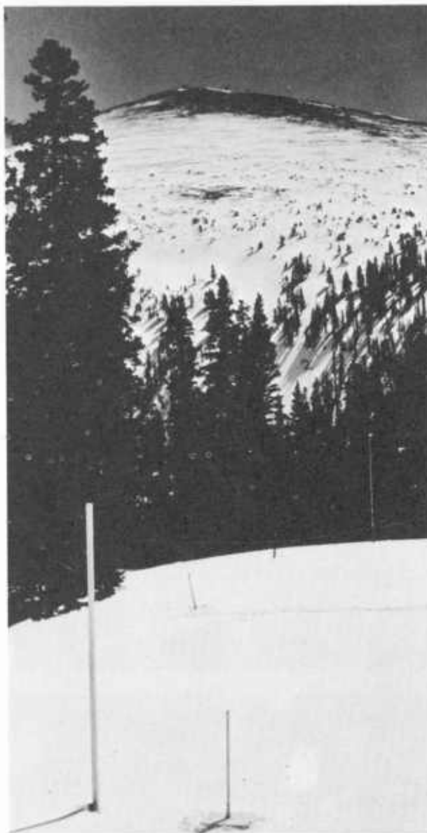
Figure 21.—Total snowstake (left), fixed to the ground, and portable snowboard (right) for measuring 24-hour, storm, or interval amounts of precipitation. Various designs are possible, but it is important that the board be made of light, nonmetallic material and that the vertical scale be sturdy.
