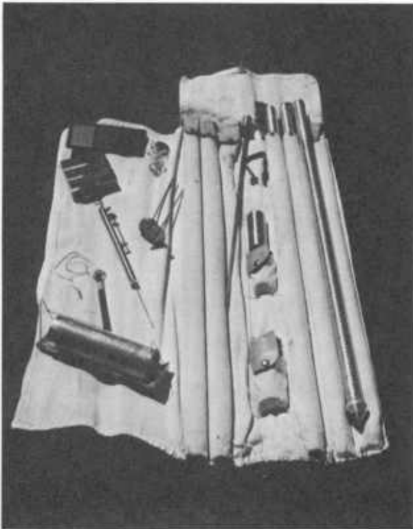
Figure 85.—Above, required and, below, optional equipment for snowpack observations. The shovel pictured here may be too light for some snow conditions.
