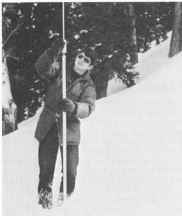
Figure 80.—The ram penetrometer is a convenient tool for snowpack observations from the surface. Using the ram, an observer can quickly determine the location of weak layers. Snowpits are required to confirm ram results.
