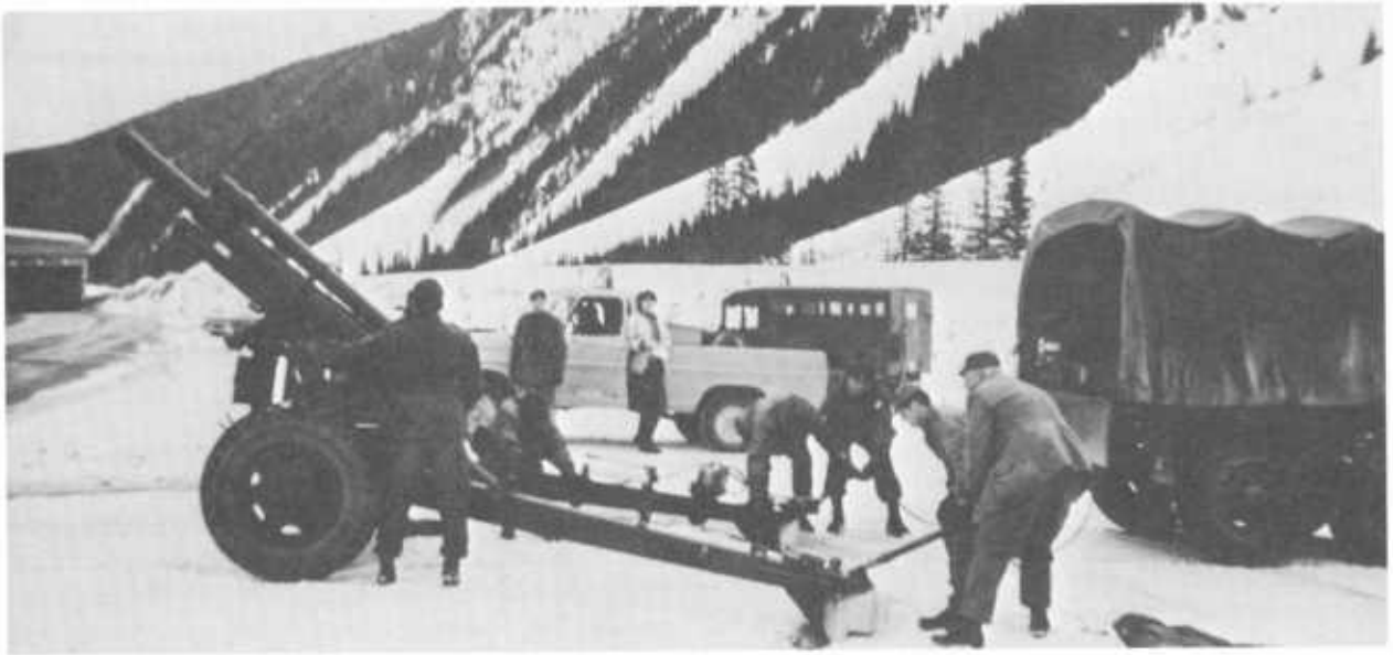
Figure 186.—Firing of 105-mm howitzer from concrete pad, Rogers Pass, B.C. A marker on the highway shed is used as reference for indirect firing.
