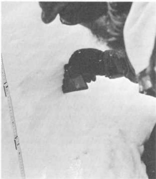
Figure 83.—Snowpit stratigraphy observation. Top left, smoothing wall with shovel; top right, brushing wall to accentuate stratigraphy; bottom left, running straightedge down wall; and bottom right, hand lens observation of snow texture.
