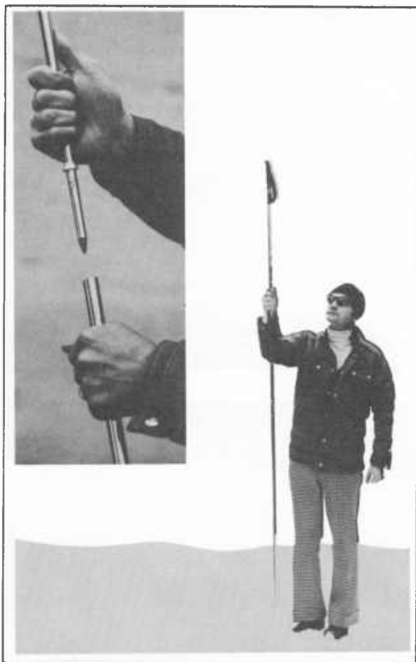
Figure 208.—One useful system for ski touring is to carry ski poles that can be assembled into probe-poles.
