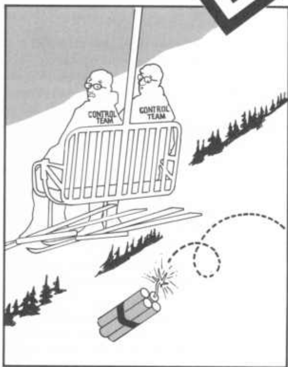
Figure 147.—Tossing charges from ski lifts entails special risks. Take special precautions against entangling charges in any of the lift equipment. All chairs should be vacant except for the blasting team. Charges should be tossed downslope and away from chairs that are moving uphill.
