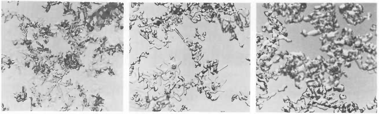
Figure 60.—Examples of grains in succeeding states of ET metamorphism. Grains are evolving toward rounded forms. (Photos by LaChapelle)
