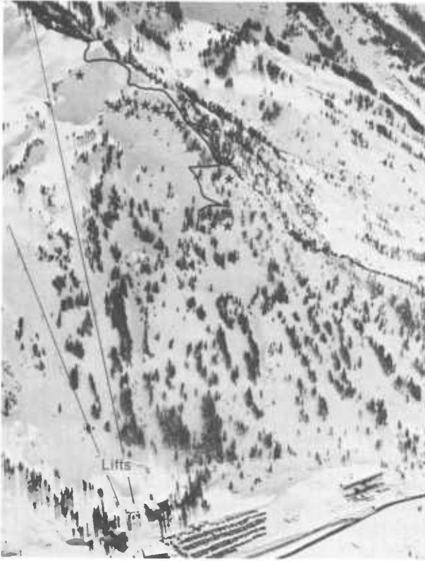
Figure 141.—Target areas along control routes at a Utah ski area. Explosives should normally be placed within the slab boundaries about halfway between the slab center and crown. If possible, the radius of influence should sweep into shaded pockets where structural weakness is likely to be most pronounced.
