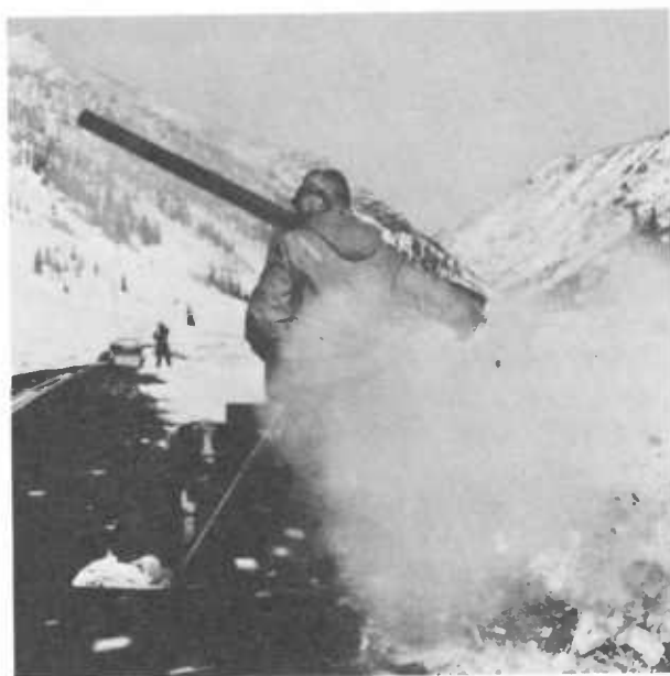
Figure 154.—Recoilless rifle, 75 mm, fired as a portable weapon from a temporary position. Gunner's ears should be protected from blast noise.
