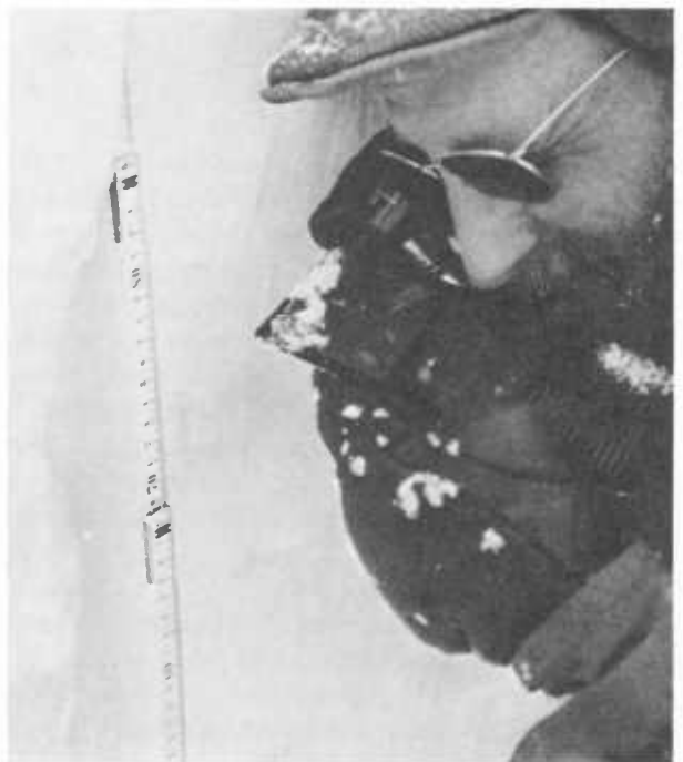
Figure 83.—Snowpit stratigraphy observation. Top left, smoothing wall with shovel; top right, brushing wall to accentuate stratigraphy; bottom left, running straightedge down wall; and bottom right, hand lens observation of snow texture.
