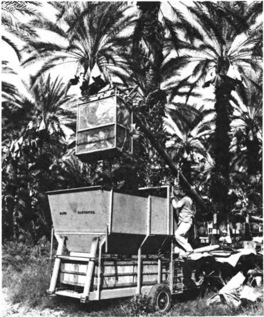
FIGURE 4. —The container with the date bunches has been lowered to a hopper containing a shaking device for removing the dates from the bunches; the dates drop into a bin underneath.
