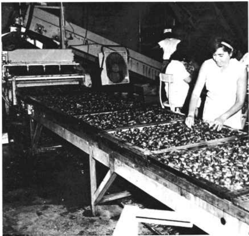
FIGURE 10. —Dry dates are trayed before introduction into the hydration chambers. The paddle wheel at the rear smooths the dates on the mesh-bottom trays and removes the excess.
