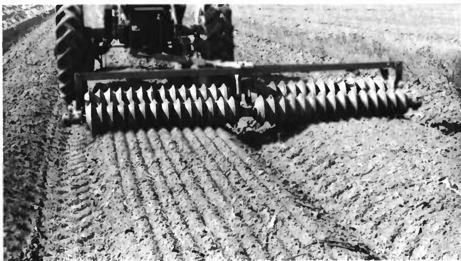
Figure 10.—Cultipacking rows after planting.
