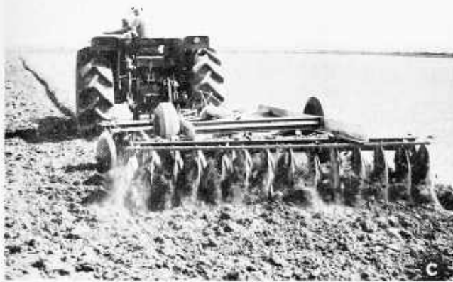
FIGURE 31.—Preparing the seedbed: A, Moldboard plow; B, field cultivator with spike-tooth harrow attached; C, disk harrow.
