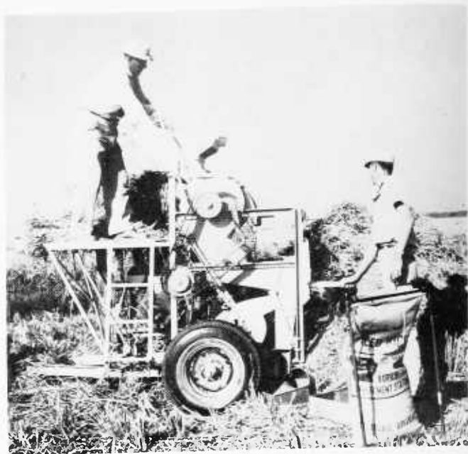
FIGURE 14.—Threshing breeder seed with a Vogel thresher.
