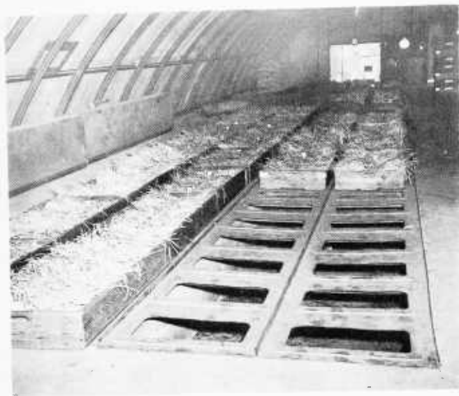
FIGURE 13.—Drying bundles of rice in trays with forced heated air.
