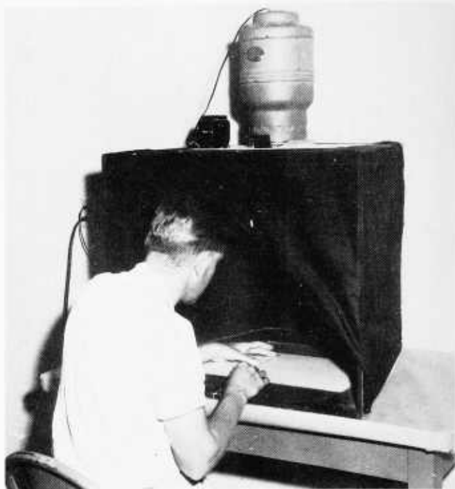
FIGURE 20.—Device for measuring rice grains and kernels.
