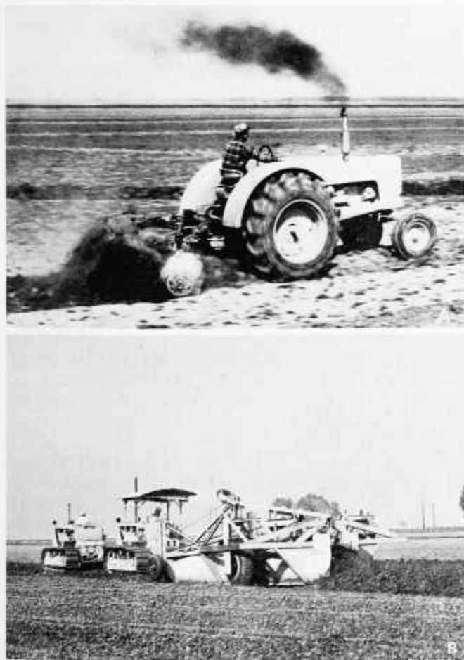
FIGURE 32.—Making levees with (A) disk, (B) pusher, and (C) plastic.
