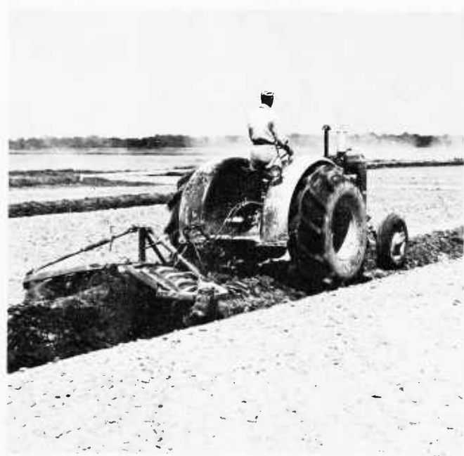
FIGURE 8.—Constructing levees in the nursery with a disk-type levee builder.
