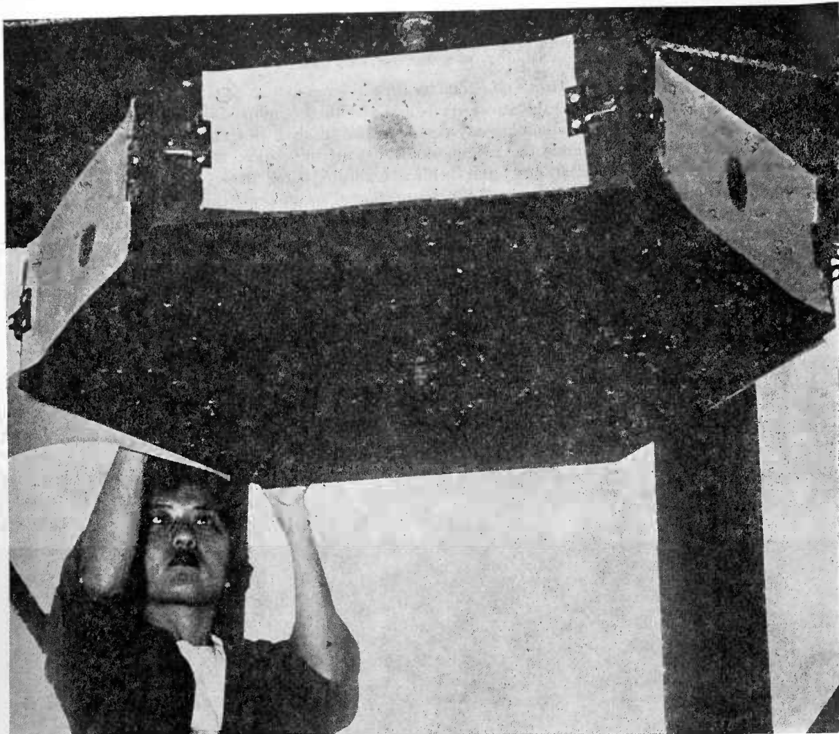
FIGURE 2.—Conducting wick tests in the olfactometer.
