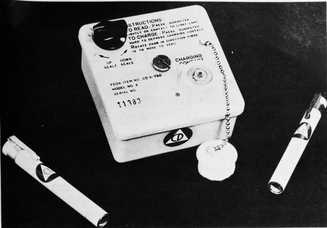
FIGURE 12.—A dosimeter measures the accumulated dosage of radioactivity.
