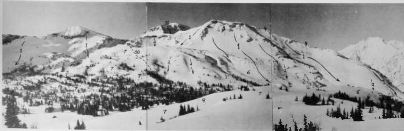
FIGURE 70.— Terrain analysis: (1) Major slide paths. (2) Lesser slide paths. (3) Narrow gully. (4) Cornice formation. (5) Convex slope. (6) Concave slope. (7) Safe area, no avalanche danger. (8) Cliffs and steep lee slopes (fracture zone). (9) Gentle, open slopes—beginner's ski area. (10) Possible lift location. (11) Arrow points to existing lift terminal just beyond pass. Almost all slopes shown are accessible from this lift. Albion Basin, Alta, Utah.
