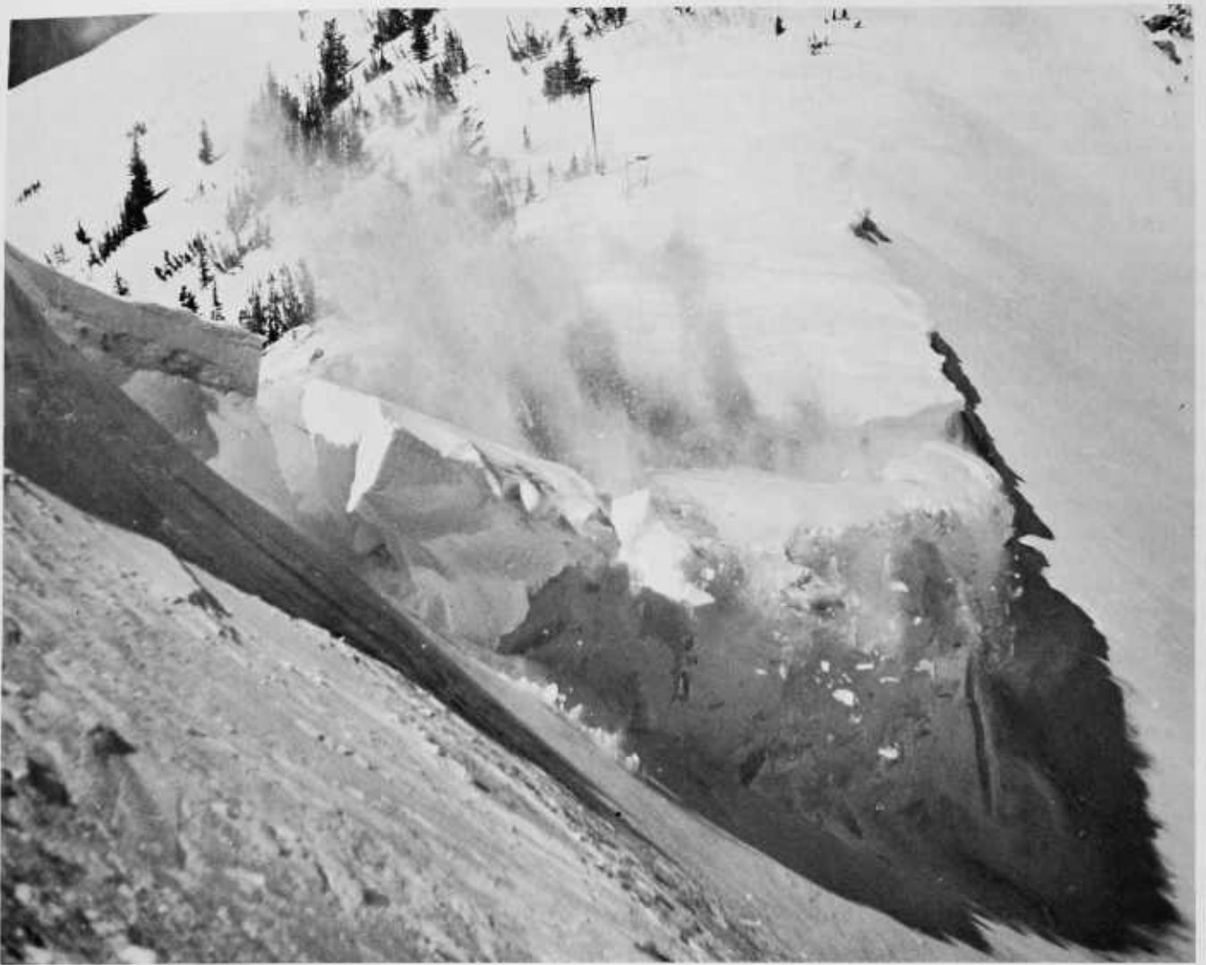
FIGURE 44.—Dynamite release of massive cornice at Twin Lakes Pass, Alta, Utah. This cornice is about 75 feet long and 25 feet high at the face. Ten shot-holes were used, spaced 8 feet apart along a straight line and drilled 6 feet deep. Each hole was loaded with two sticks of 40 percent gelatin.
