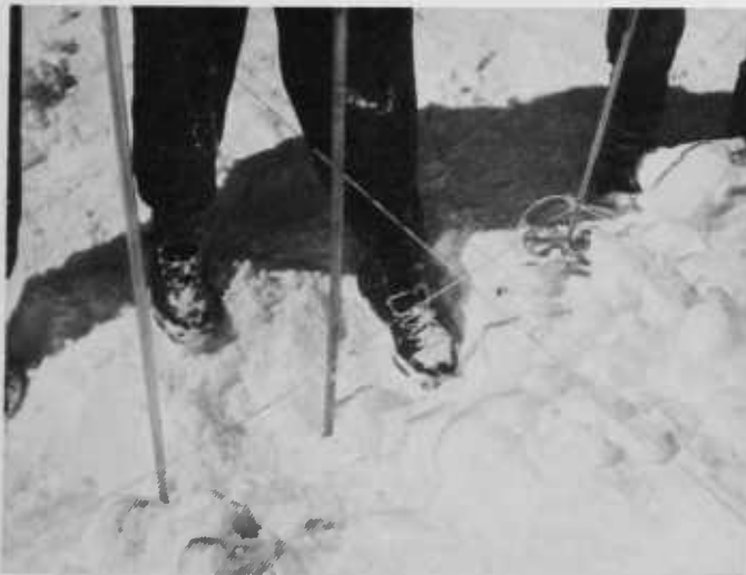
FIGURE 68.—String marker method used to guide probing operations. The string shown tied to the ski pole is moved one foot ahead after the complete line has been probed. The other string stays in place as a permanent marker for the area probed.
