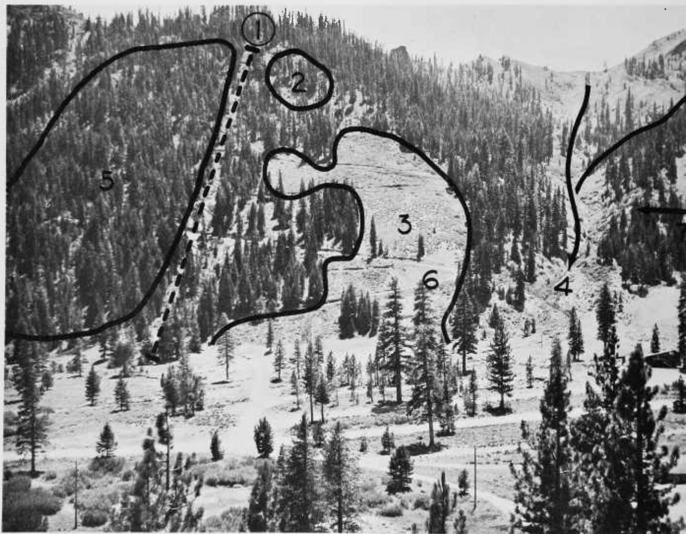
FIGURE 72.—A new ski slope in the process of development. (1) Lift line partially cleared. (2) Only observed avalanches on the mountain originate in this area of scattered timber. (3) A natural clearing. (4) An avalanche gully flanking the new area. (5) Area of heavy timber, very steep but completely stable. (6) Construction road. Switchbacks screened behind timber. Arrow at right, prevailing wind direction. The slope faces north.
