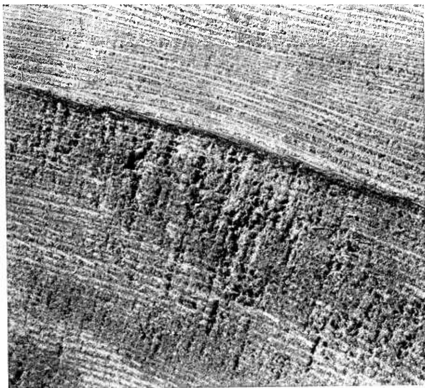
FIGURE 14.—End-grain surfaces of spruce lumber showing fiber breakage caused by compression failures confined to the part below the dark line. Slightly magnified.
