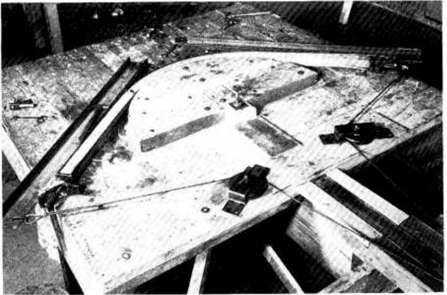
FIGURE 68.—Apparatus for bending heavy members. The end blocks of the metal strap are equipped with reversed levers made from I-beams, which prevent the end blocks from overturning and sliding off, help to regulate end pressure, and reduce the tendency of the stick to assume reverse or back bends near the ends.
