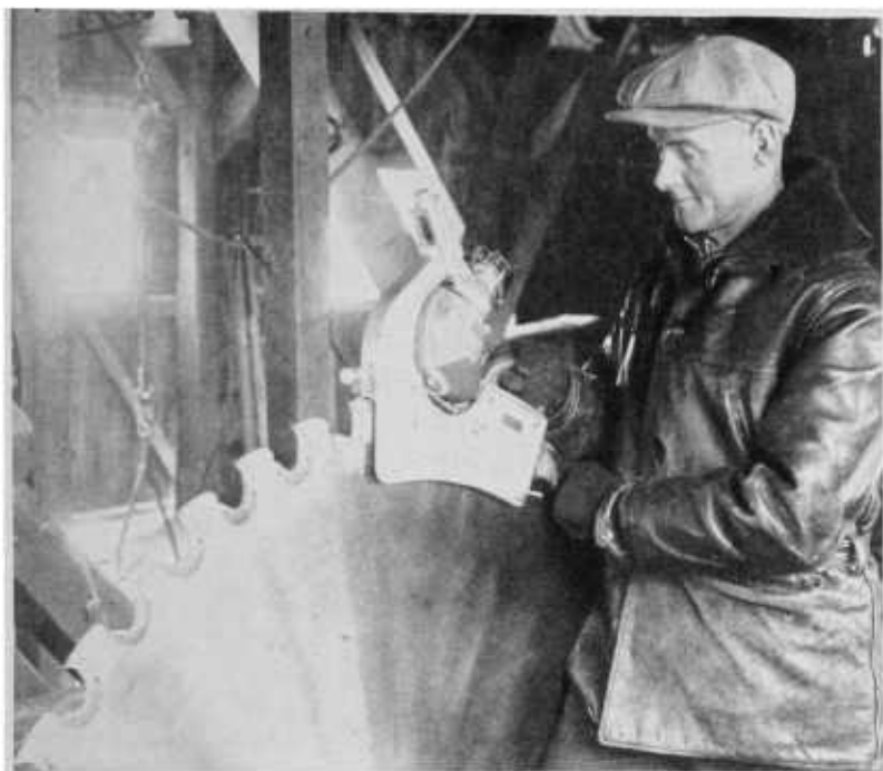
Figure 8.—Tooth-sharpening machine with powered emery wheel.
