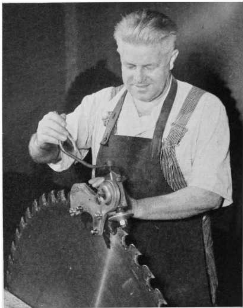
Figure 7.—Tooth-sharpening machine using handcranked wheel faced with file segments.
