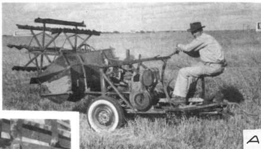
Figure 5.A, Two-reel stripper used in central Texas to harvest seeds of some native and introduced grasses; most often used on little bluestem. B, Another view showing belted slat of larger reel approaching and pushing seedstems against the smaller reel.
