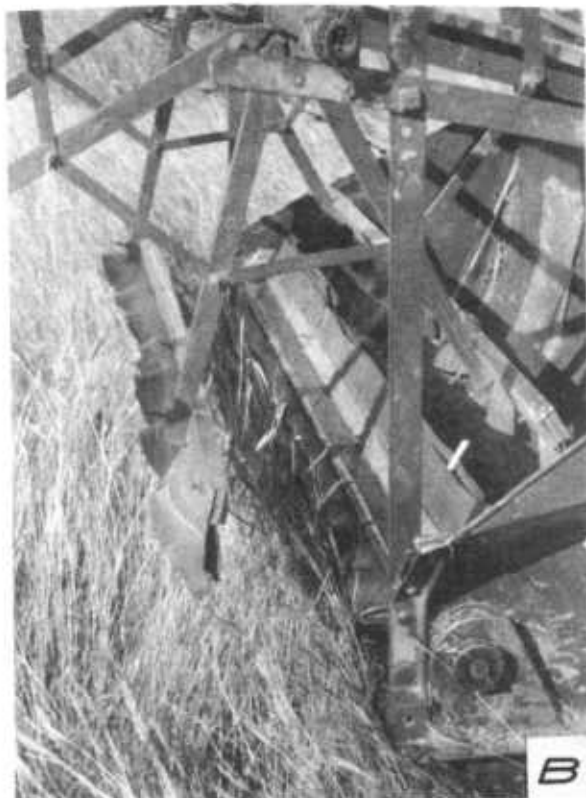
Figure 6. Dublin topper for harvesting seedhay of native grasses; the machine shown is mounted on a road truck.
