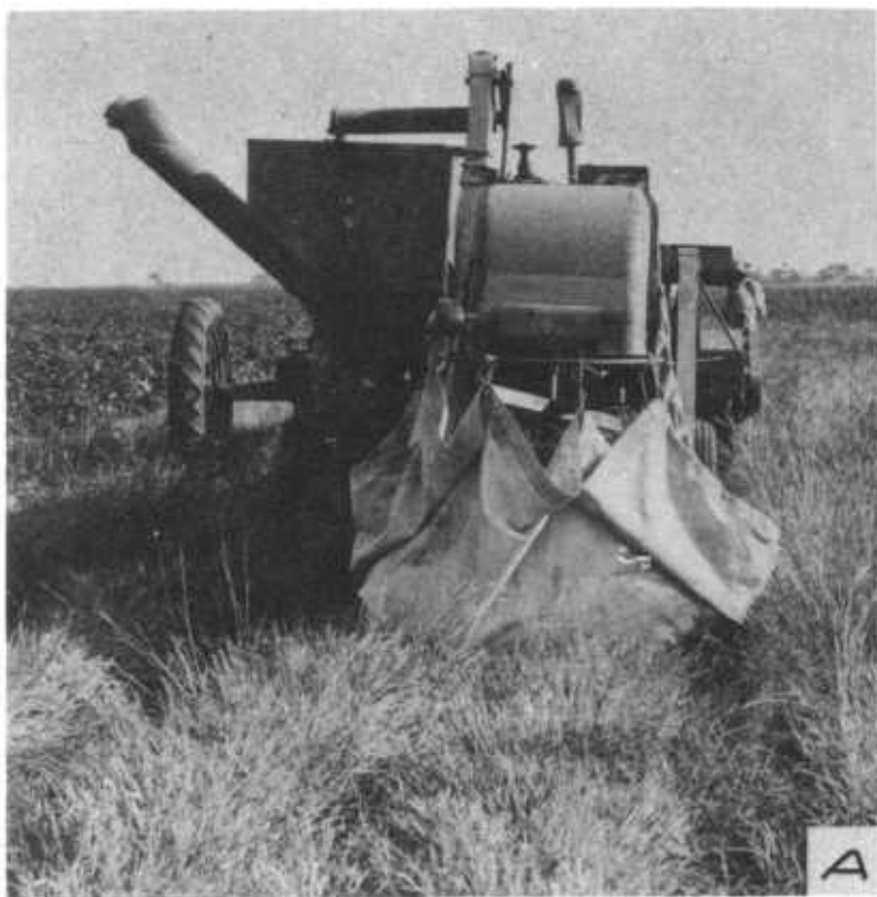
Figure 4. A, One way of collecting tailings of King Ranch bluestem that contain good seeds; the canvas is hung from the hood. B, Combining Dallisgrass from windrows in Louisiana.
