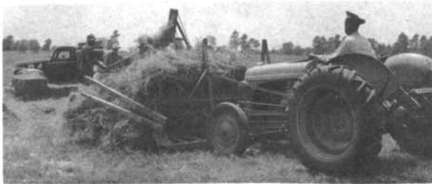
Figure 8. Using a buncher or sweep rake to carry hay to the machine.
