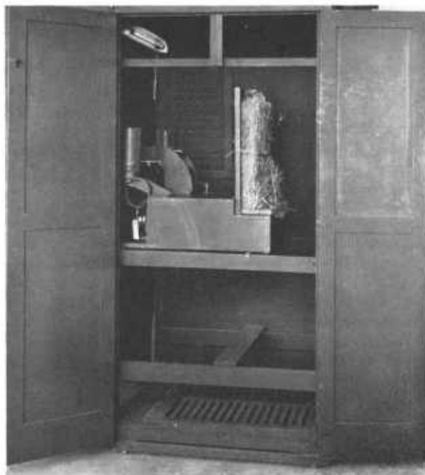
FIGURE 21.—Another early type of disk colorimeter (Keuffel & Esser) designed to measure areas of hay 14 inches in diameter. A side view is shown, with hay sample in place. The entire instrument is enclosed in a small portable darkroom cabinet (note rollers on bottom of platform). After the hay sample is placed in position the double doors are closed, and the operator goes around to the front of the instrument where he works behind a dark curtain that cuts off light from the room in which he is working. This instrument is in regular use today for hay-color measurement.
