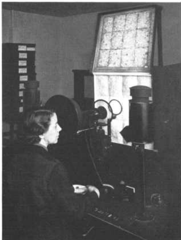
FIGURE 20.—Early disk colorimeter designed to replace spinning of disks by a spinning optical part, and provide for sample and disk illumination within an instrument. This instrument (Keuffel & Esser) provides for measuring an area of 4 inches in diameter behind the black ring. This instrument is in regular use for measuring cotton color.
