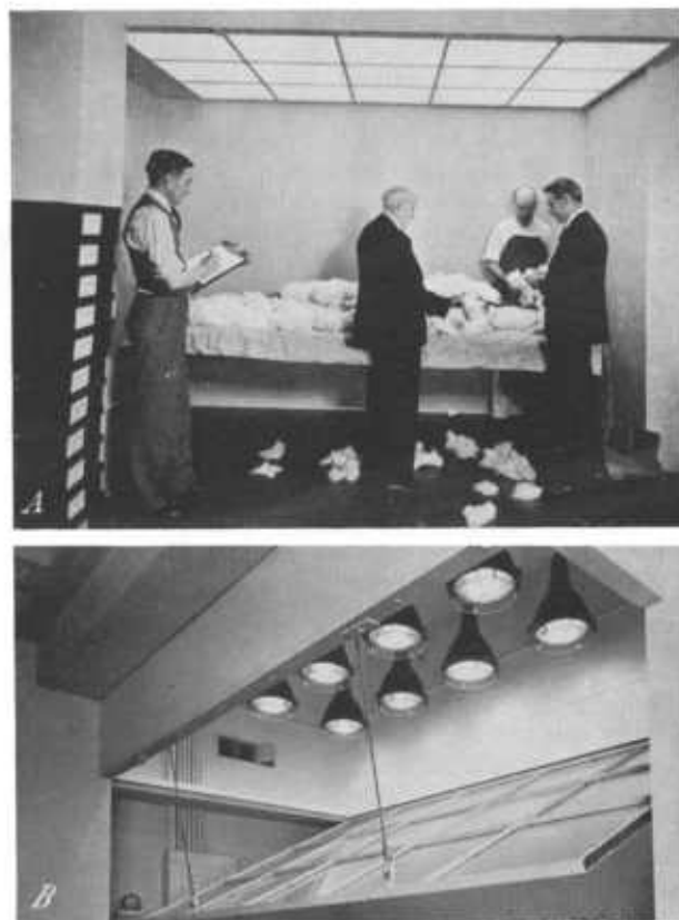
FIGURE 44.—Artificial daylight installation used in experiments to determine specifications necessary for satisfactory artificial daylighting for cotton and other agricultural commodity grading: A, Light in use; B, lamps provided with filters of Corning daylight glass, and construction of the diffusing glass panel that produces a skylight effect.
