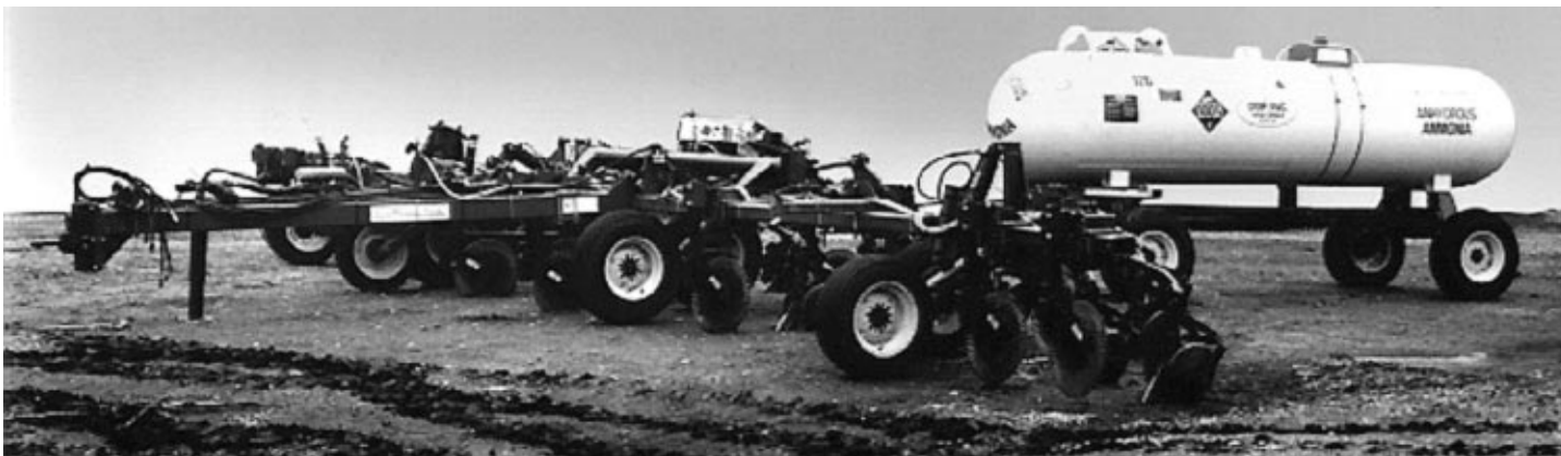
Fertilizer dealers typically put the anhydrous ammonia in 1,000 gallon "nurse" tanks for delivery to farms, where the tanks are hooked to application equipment. This application equipment spans 16 rows and injects anhydrous ammonia 8 inches underground.
